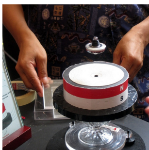
Figure 2.1: On the left magnetic levitation stabilized using rotation is shown [8]. On the right Pseudo-levitation of two permanent magnets on a guide rod is shown [9].
