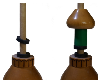
Figure 2.1: On the left magnetic levitation stabilized using rotation is shown [8]. On the right Pseudo-levitation of two permanent magnets on a guide rod is shown [9].
