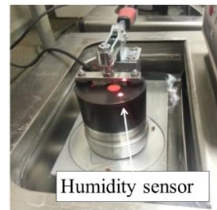
(d) Placing the humidity sensor (with slightly higher temperature (20.3 °C)) on the sample holder
