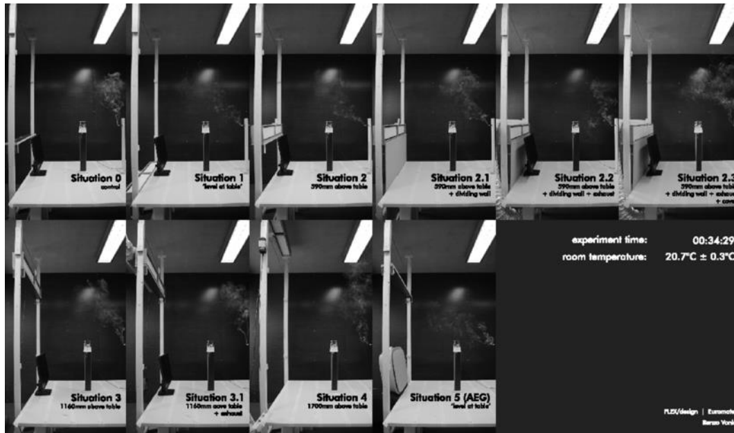
Figure 34: Snapshot of video compilation demonstrating air flow direction for each scenario described in chapter 5.4.1
