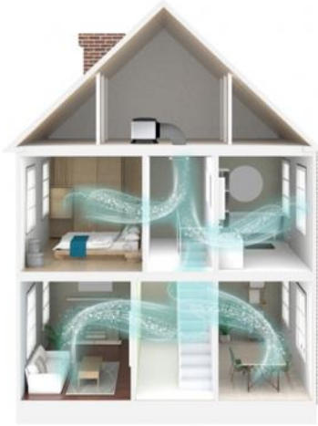
Figure 19: PIV system placed in the attic of a residential building (Envirovent, n.d.)
