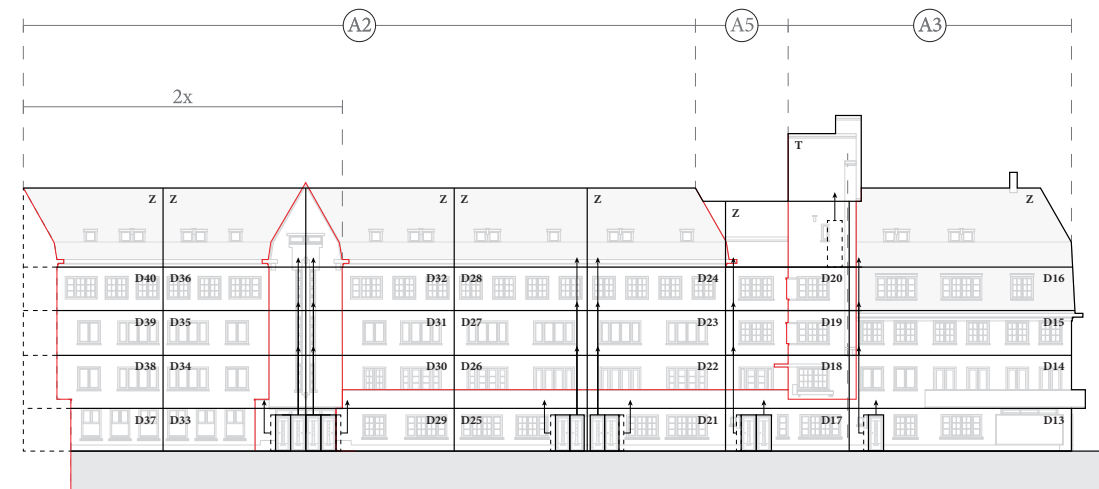
Figure 50: The grid of de dwellings behind the facade on the west corner of the Churchill-laan 1:5000 (Kroes, 2024)
