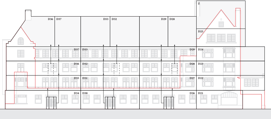
Figure 44: The grid of the dwellings behind the facade on the Gerret van der Veen straat 1:3500 (Kroes, 2024)
