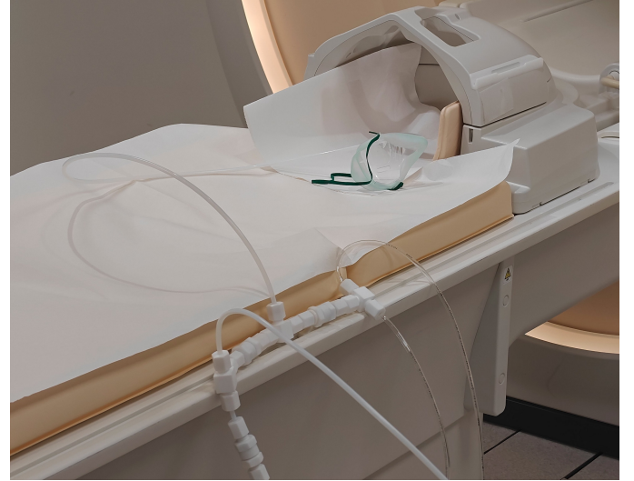
Fig. 6: Position of the vacuum-switch in the MRI room. Shown here is the position at the bore entrance. The picture does not show the table inside the MRI bore, which is the case for the test.
