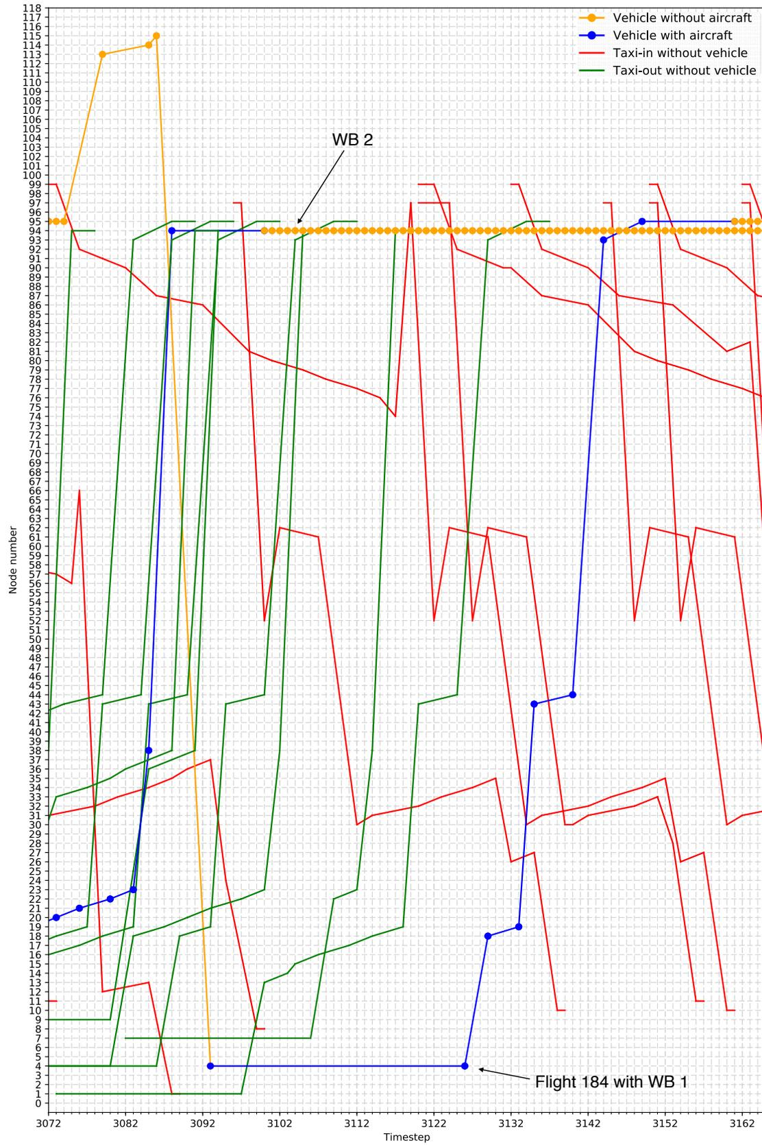
Figure C.2: Time-space graph of in-bound and out-bound taxiing traffic at the surface of AAS using two WB AGVs.
