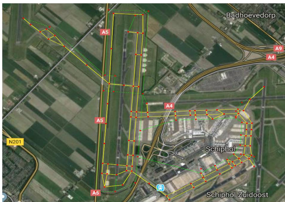
Figure 4.13: The aircraft taxiing network (indicated with the yellow lines) and the service roads (indicated with the dotted green lines). The distances between the nodes are the real taxiing distances obtained from Roling [2009]
