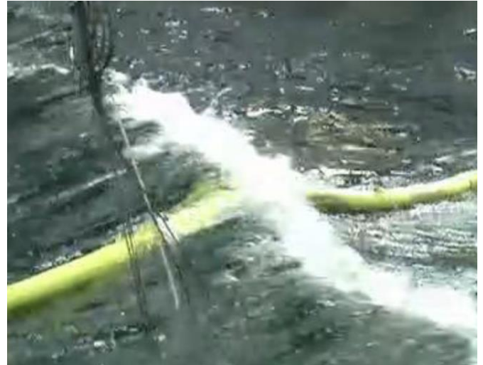
Figure 3 – Visually observed overtopping event during scale model tests conducted by Mocean at MARIN test facilities in 2015. (Image courtesy of The Ocean Cleanup)
