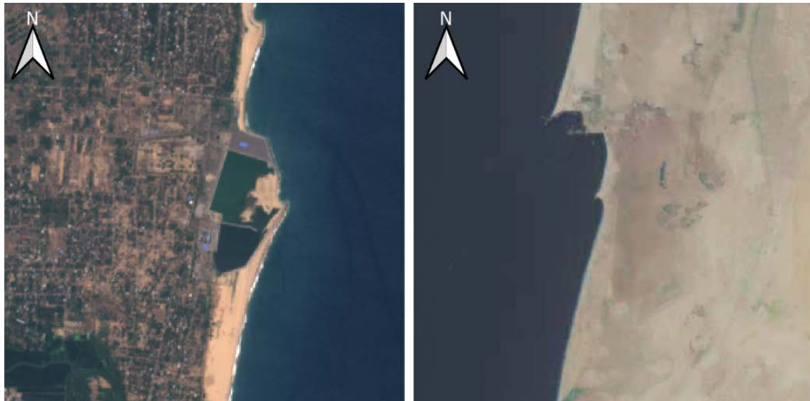
Figure 2.24: Left: Harbour siltation, Oluvil Port, Sri Lanka; right: updrift accretion, downdrift erosion, Port of Nouakchott, Mauritania. Images from Sentinel-2 cloudless by EOX IT Services GmbH are licensed under CC BY 4.0.
