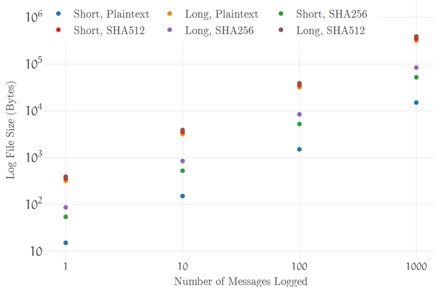
Figure 11: Scatter plot of the log file size in bytes after logging the designated number of lines. The horizontal axis is base 10 logarithmic.
