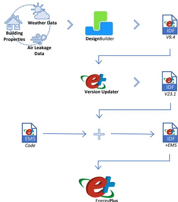
Figure 25: BPS Model Software Workflow
