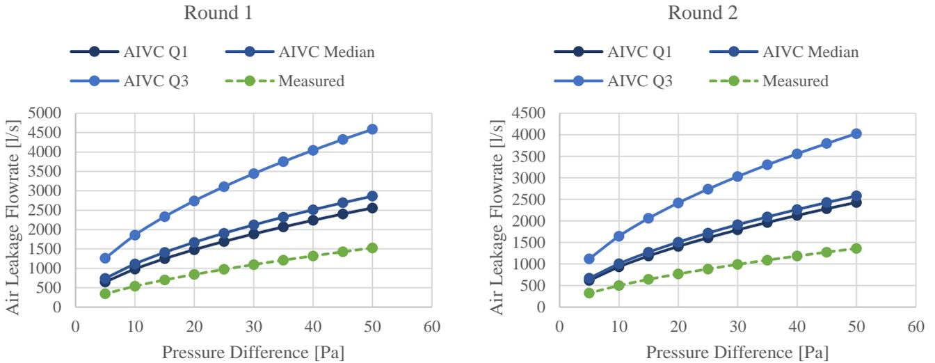
Figure 84: Measurements and AIVC Estimates of Building Air Leakage
