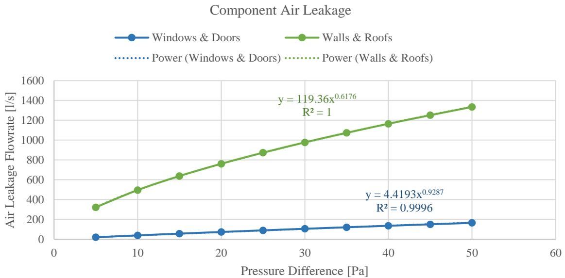
Figure 19: Component Air Leakage Characteristic Non-normalized Power Law Equations
