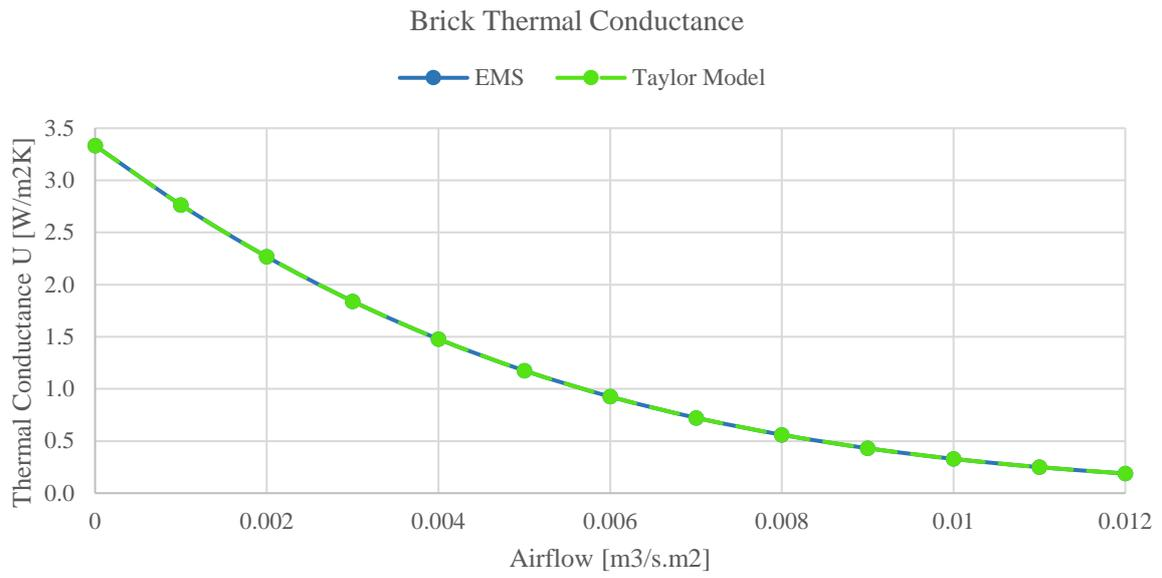
Figure 87: Single-layered Construction's Brick U-value - EMS vs. Taylor Model
