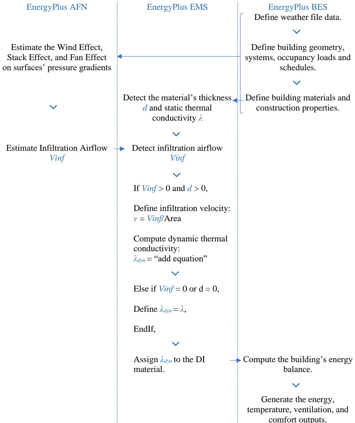
Figure 28: Flowchart of the EnergyPlus' EMS algorithm logic for DI System Modelling
