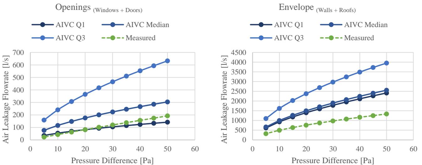
Figure 85: Measurements and AIVC Estimates of Component Air Leakage
