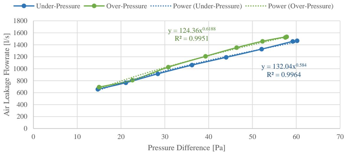
Figure 79: Round 3 Under-Pressure and Over-Pressure Power Law Equations
