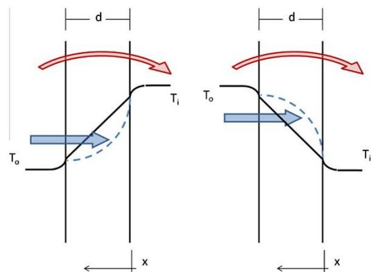
Figure 8: Airflow's Impact on Constructions' Temperature Distribution (Solupe & Krarti, 2014)
