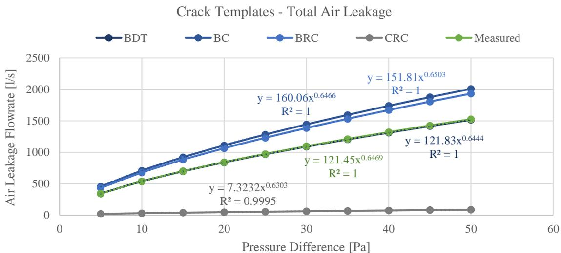
Figure 86: Building's Air Leakage Behavior - Measurements vs Crack Templates
