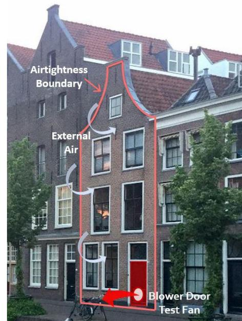
Figure 16: Fan-pressurization Test Setup
