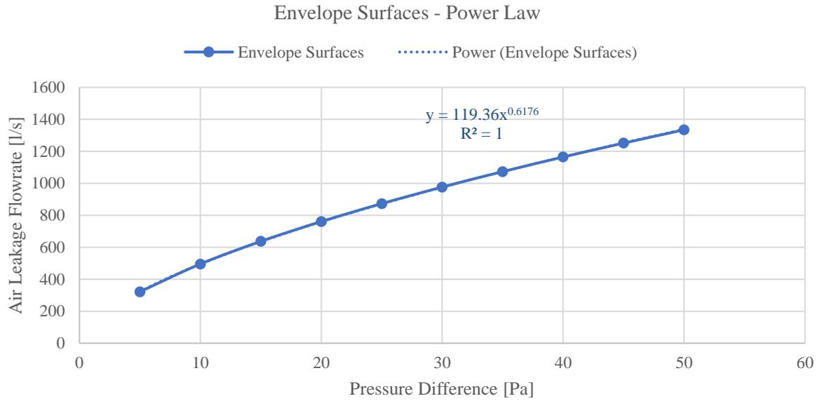
Figure 83: Envelope Surfaces' Fitted Power Law Equation
