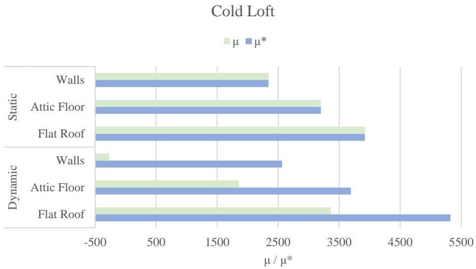
Figure 35: Morris SA Metrics ( $\mu/\mu^*$ ) under Cold Loft Case – Under-pressure Operations
