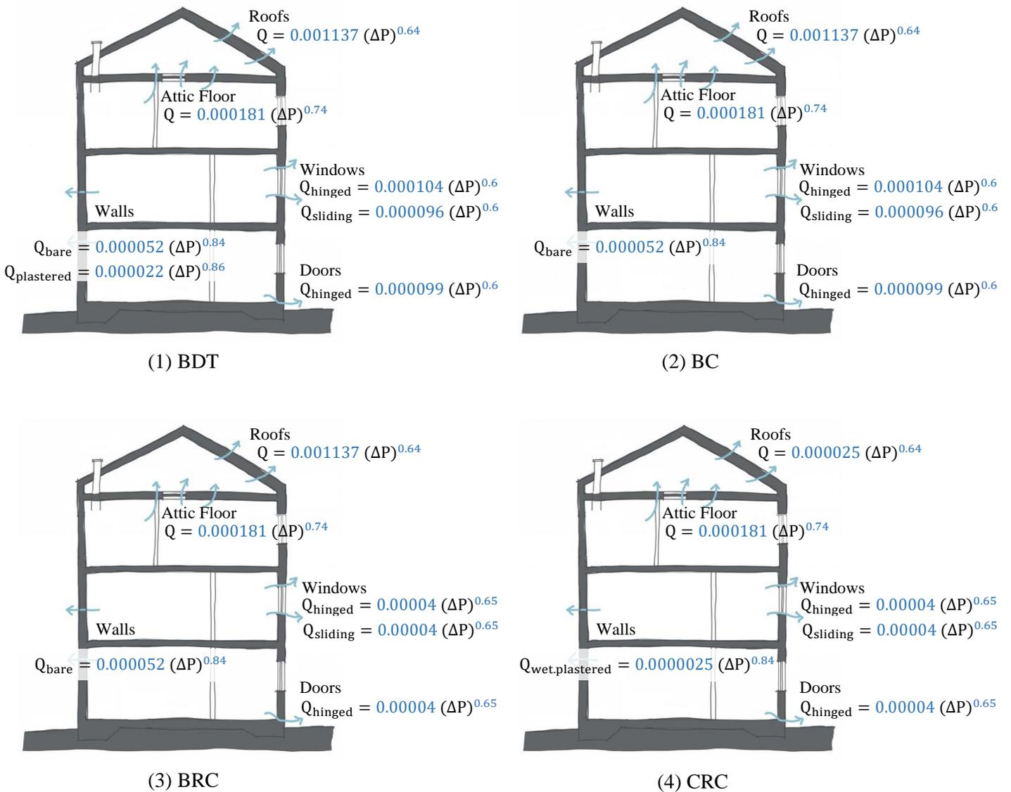
Figure 26: Air Leakage Model's Crack Templates
