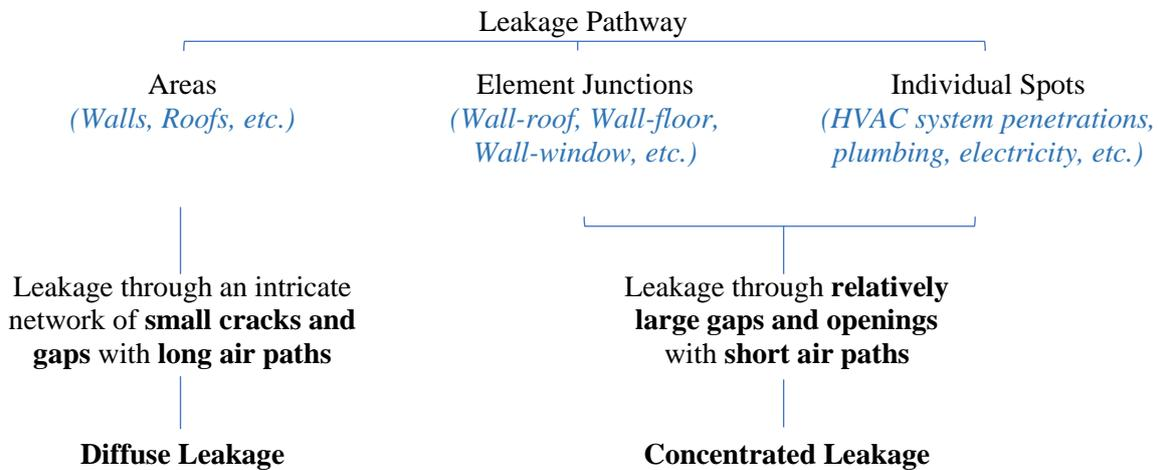
Figure 5: Air Leakage Classification
