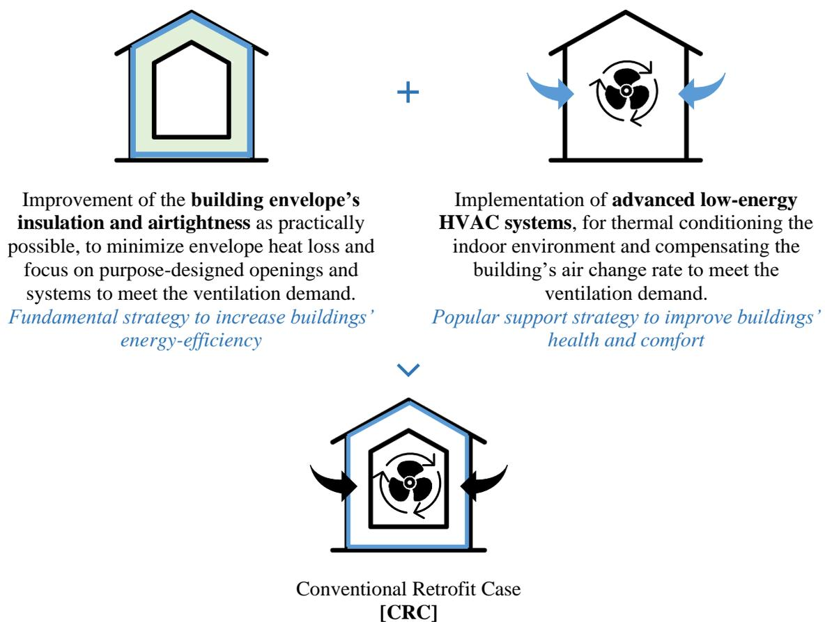
Figure 12: Conventional Retrofit Case (CRC) Components
