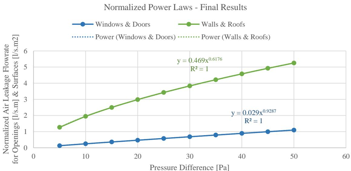
Figure 20: Component Air Leakage Characteristic Normalized Power Law Equations
