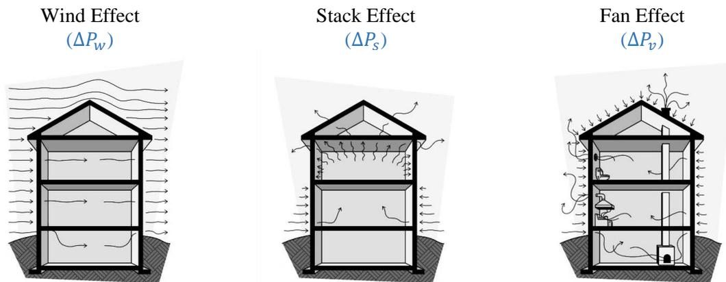
Figure 3: Air Leakage-driving Pressure Components (NAIMA Canada, n.d.)
