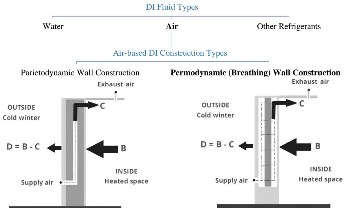
Figure 10: Air-based DI Construction Types (Fawaier & Bokor, 2022)
