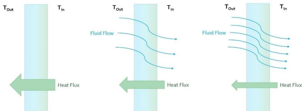
Figure 9: Fluid Flow's Impact on the Envelope Construction's Heat Flux
