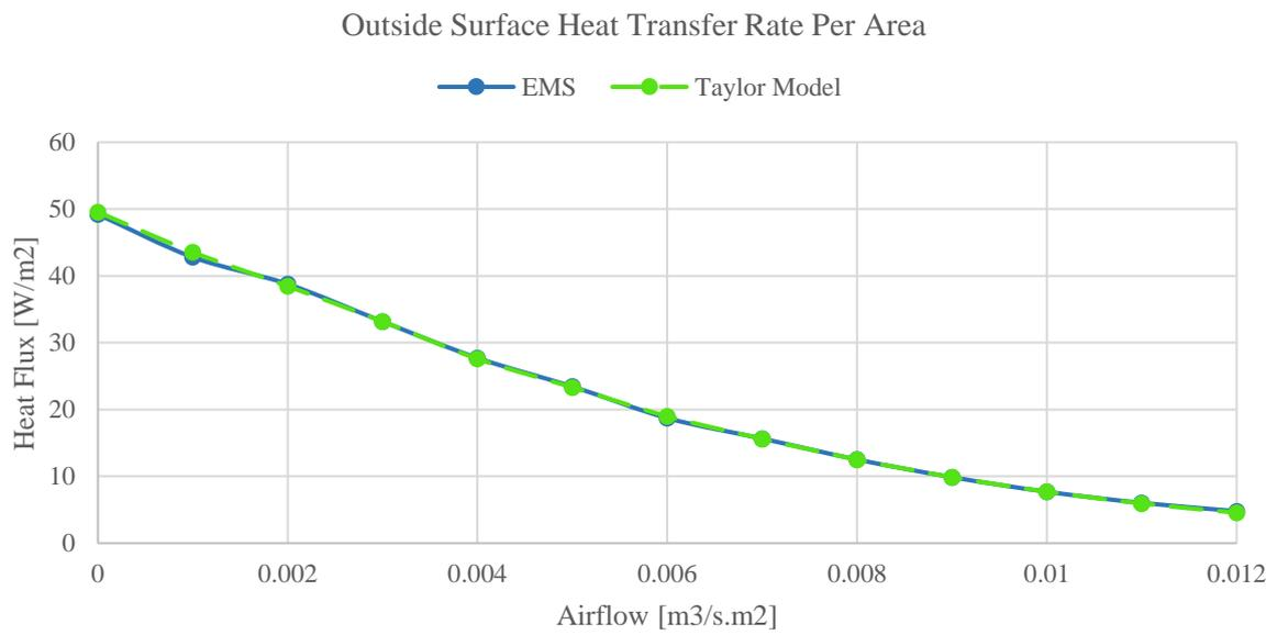
Figure 88: Single-layered Construction's Outward Heat Flux - EMS vs. Taylor Model
