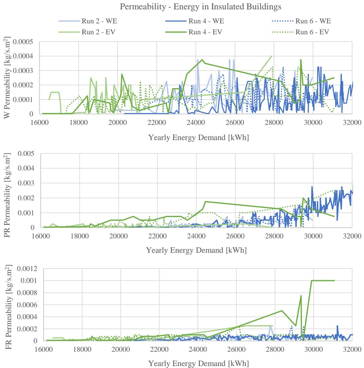
Figure 63: Permeability vs Energy - Insulated Buildings
