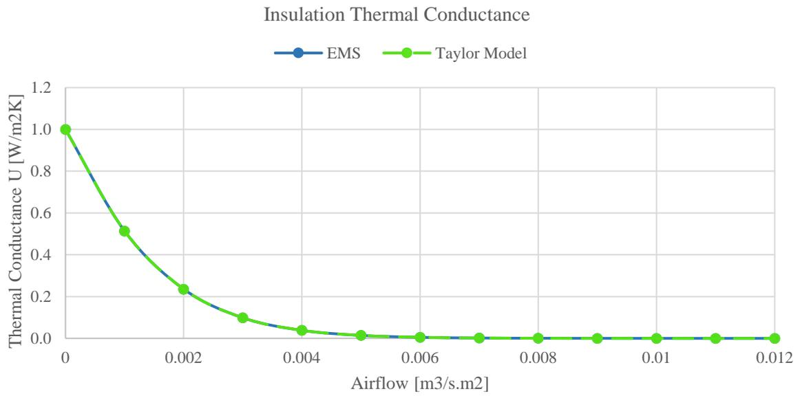
Figure 90: Multi-layered Constructions' Insulation U-value - EMS vs. Taylor Model
