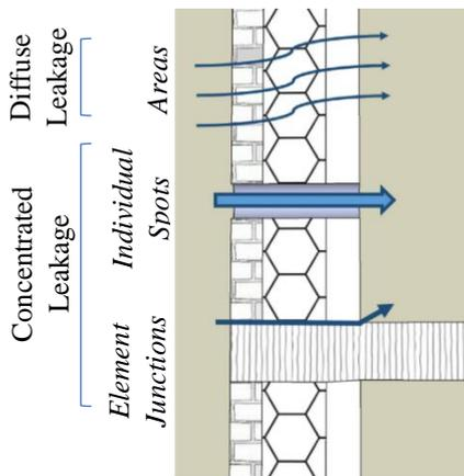
Figure 6: Air Leakage Pathway Types (Prignon & Van Moeseke, 2017).
