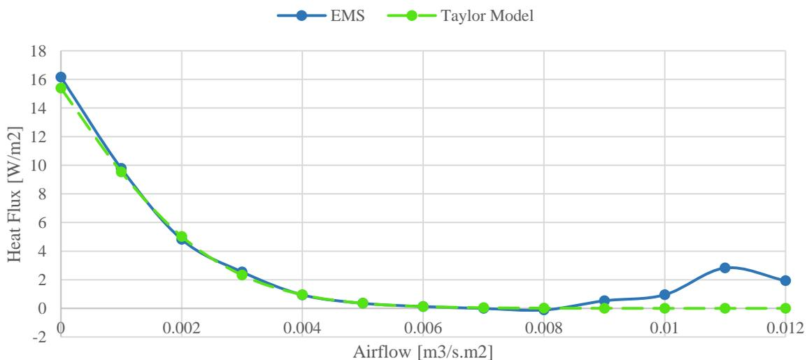
Figure 91: Multi-layered Construction 1's Outward Heat Flux - EMS vs. Taylor Model
