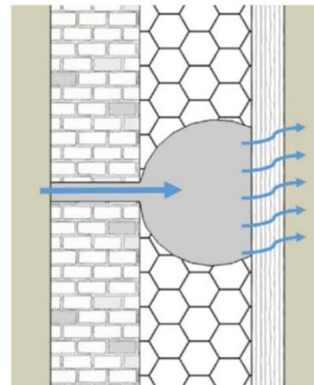
Figure 7: Air Leakage Hybrid Pathway (Prignon & Van Moeseke, 2017).
