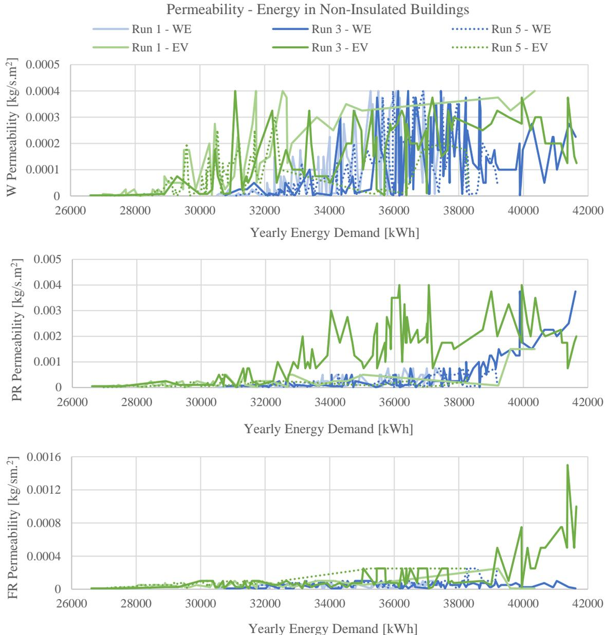
Figure 64: Permeability vs Energy - Non-insulated Buildings
