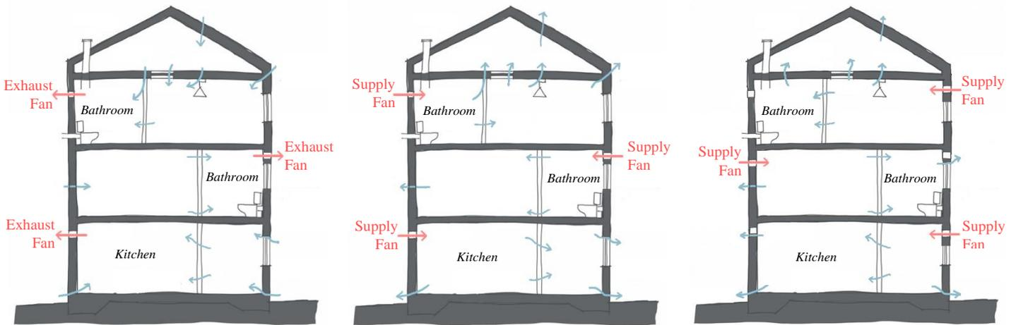
Figure 62: Building Air Movement under Exhaust Ventilation in Wet Rooms (left), and Supply Ventilation in Wet Rooms (middle) and Living Spaces (right)
