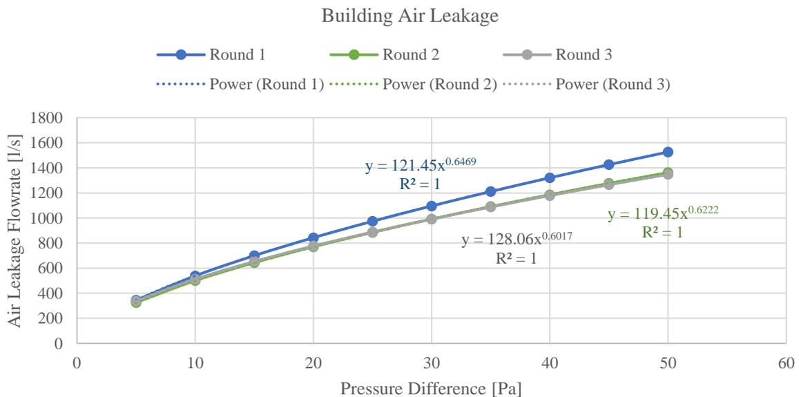
Figure 18: Building Air Leakage Characteristic Power Law Equations
