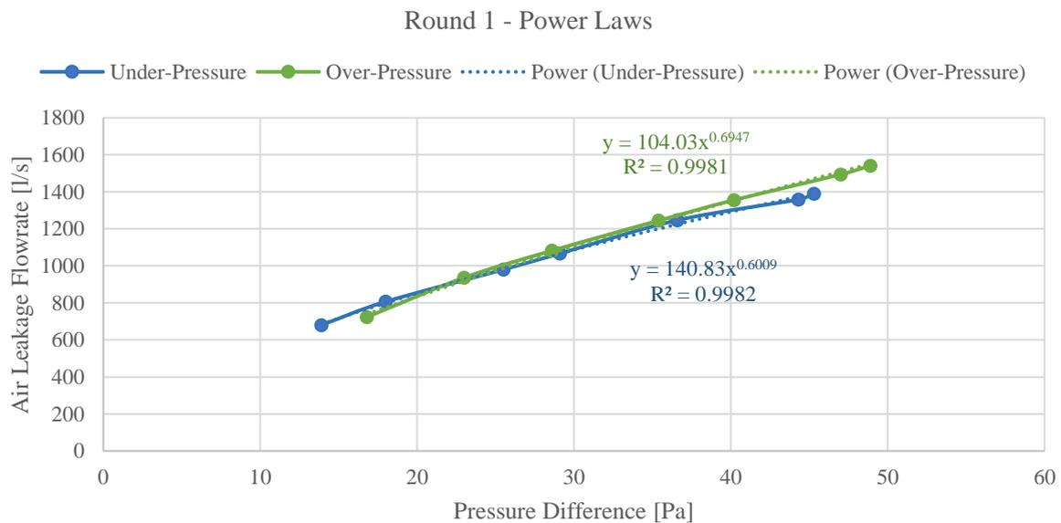
Figure 75: Round 1 Under-Pressure and Over-Pressure Power Law Equations
