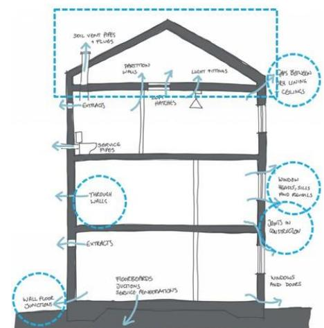
Figure 4: Air Leakage Main Pathways
