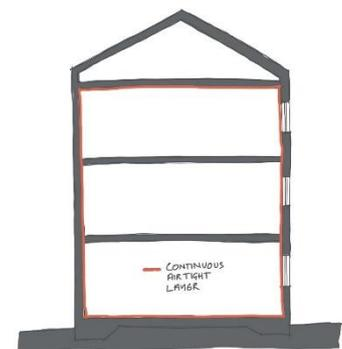
Figure 2: Airtightness, a Building Property (Airtightness, n.d.)
