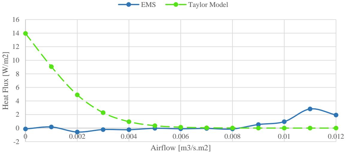
Figure 92: Multi-layered Construction 2's Outward Heat Flux - EMS vs. Taylor Model
