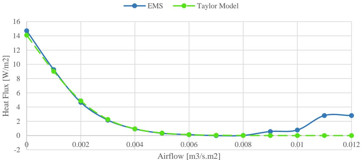
Figure 93: Multi-layered Construction 3's Outward Heat Flux - EMS vs. Taylor Model
