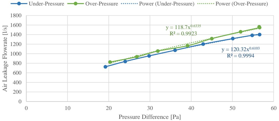
Figure 77: Round 2 Under-Pressure and Over-Pressure Power Law Equations
