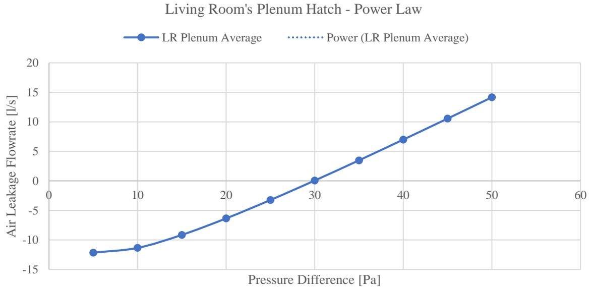
Figure 82: Living Room Plenum Hatch's Fitted Power Law Equation
