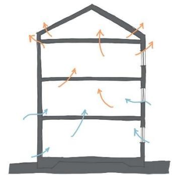
Figure 1: Air Leakage, a Physical Phenomenon (Airtightness, n.d.)
