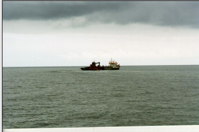
Figure 3.1 Trailing suction hopper dredger extraction sand from the North Sea bed, source: RIKZ
