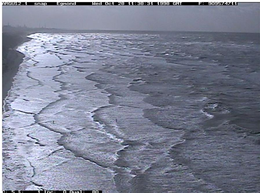
Figure 3.4 Dissipation of wave energy as a result of breaking off the coast between Egmond aan Zee and IJmuiden, as seen from the argus video station 'Coast3D' (see also [www.wldelft.nl/argus](http://www.wldelft.nl/argus)).
