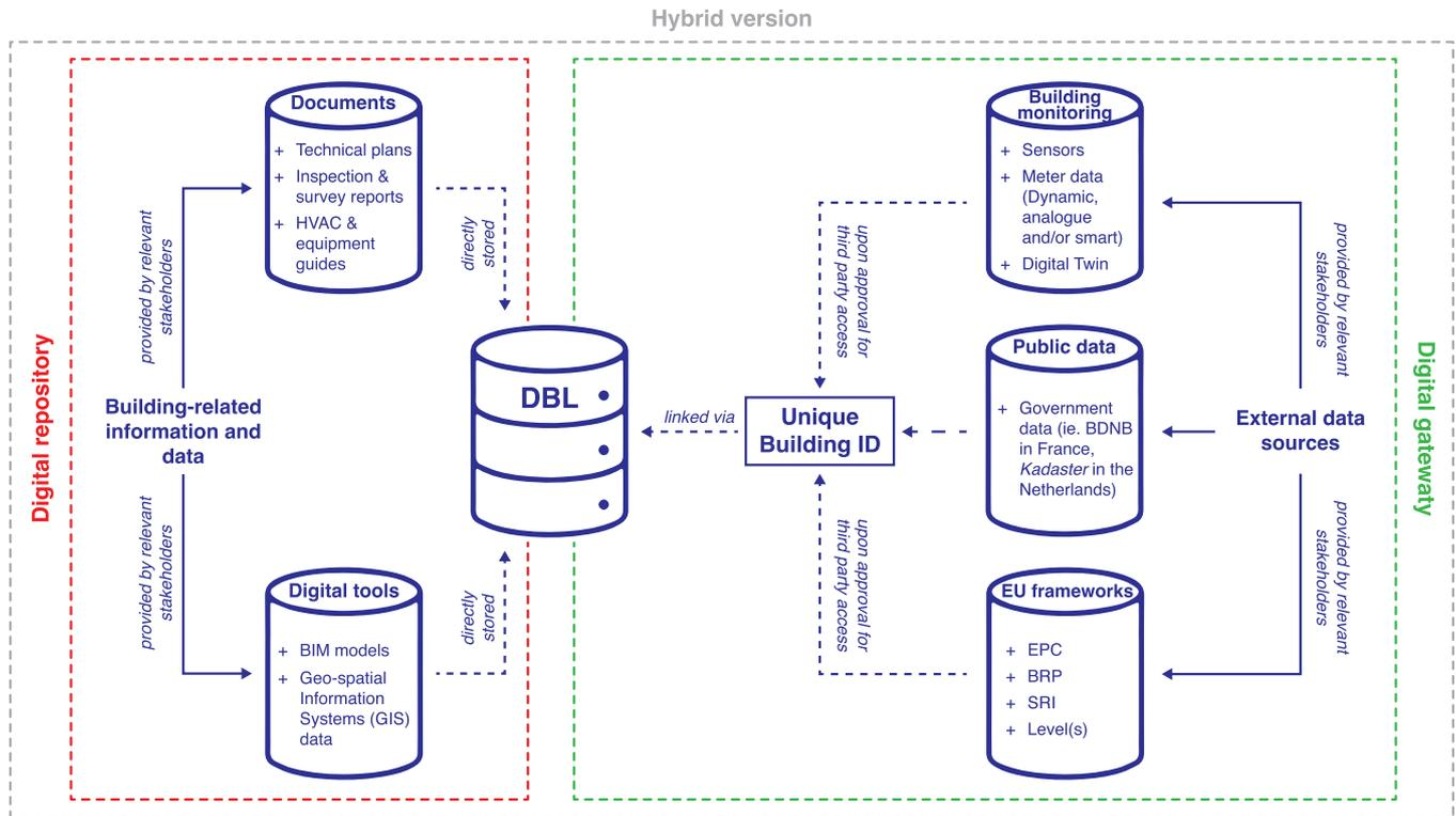
Fig. 3. The ways in which building data can be stored in and/or linked to the DBL (Own illustration).
