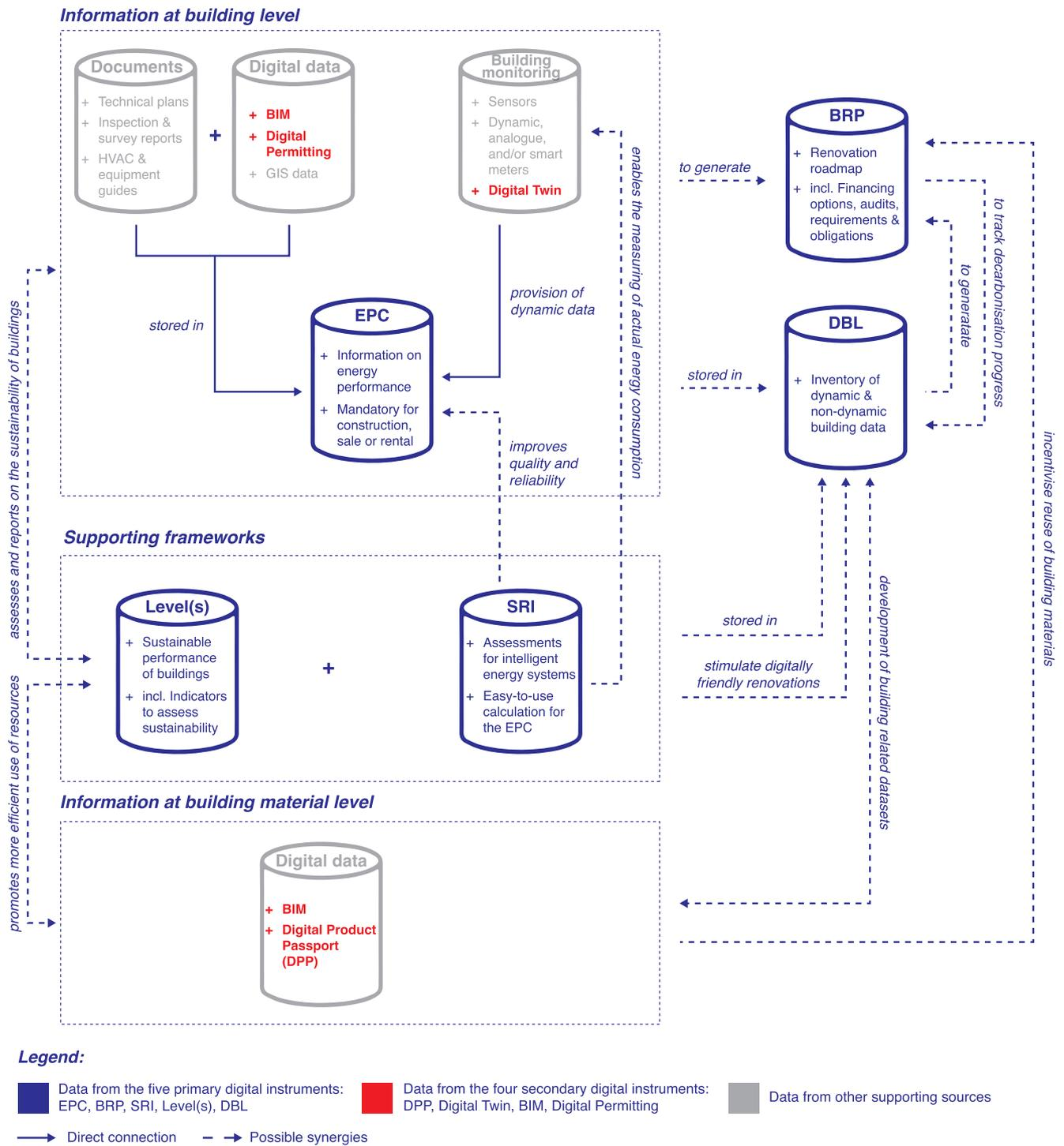
Fig. 4. The proposed Digital Energy Renovation Framework (Own illustration).
