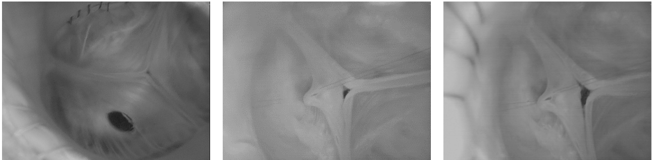
(a) Subject 2 with a punched valve (50 mmHg) (b) Subject 3b with medium insufficiency (40 mmHg) (c) Subject 3b with large insufficiency (50 mmHg)
