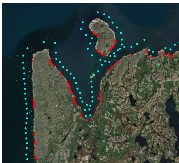
Figure 3.4: Satellite imagery overlain with SDS transect origins that have identified the coastline as beach (blue) and visually confirmed unconsolidated coastline. These discrepancies are common in this region, where granite cliffs and boulders dominate the littoral zone
