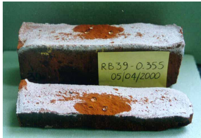
FIGS. 4.12/4.13 Salt accumulation beneath the layer treated with a water repellent (left) and subsequent spalling of the treated part (right) during a laboratory test / Photos: B. Lubelli
