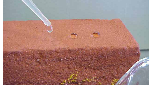
FIG. 4.19 Method for the assessment of effectiveness of water repellent treatment: beading effect / Photo: B. Lubelli
