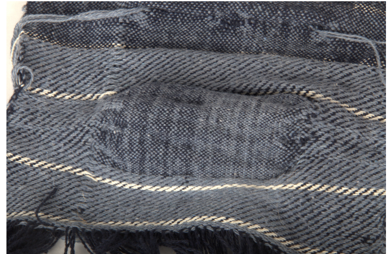
Figure 181: Top view of resulting fabric with embedded dome
