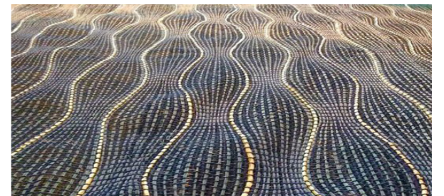
Figure 32: Fabric of which the warp threads have been curved with a fan reed (Cnaani & Sterman, 2023)
