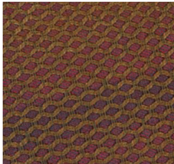
Figure 28: The backside of a bedford cord, where the floats can be seen (Shenton, 2014)
