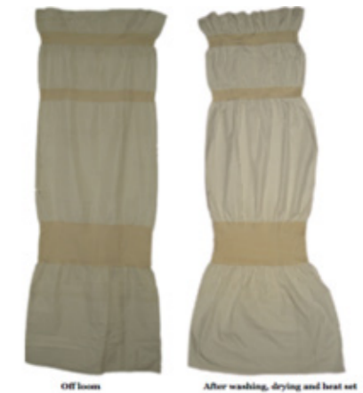
Figure 18: The shape of the fabric once taken off the loom (left) and once washed, dried and heat set (right) (Hashish, 2014)
