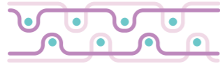
Figure 64: Illustration of a multi-layer weave structure showing how the weft threads are placed stacked on top of each other
