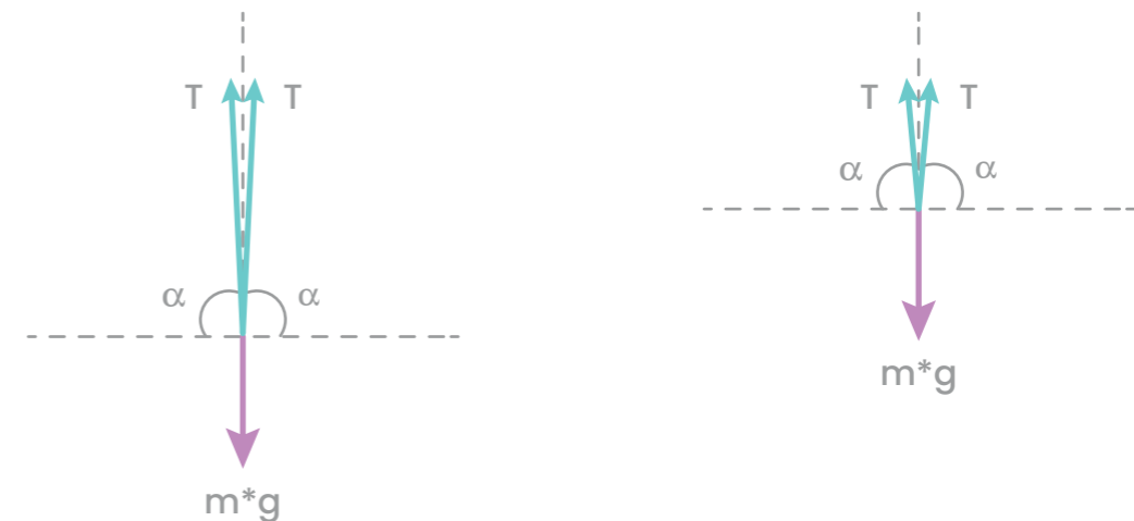
Figure 137: Visual showing how the angle barely changes when the weight is pulled up
