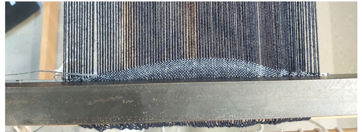
Figure 188: Picture showing a fell that has become strongly curved due to the interlacement of discontinuous weft threads
