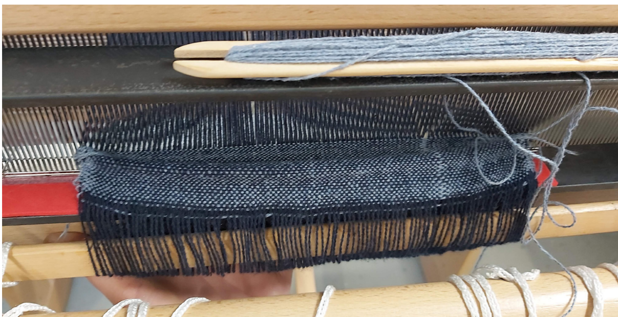
Figure 191: Picture showing how two full weft rows allowed the fabric to be flattened enough for the clamp to press down on
