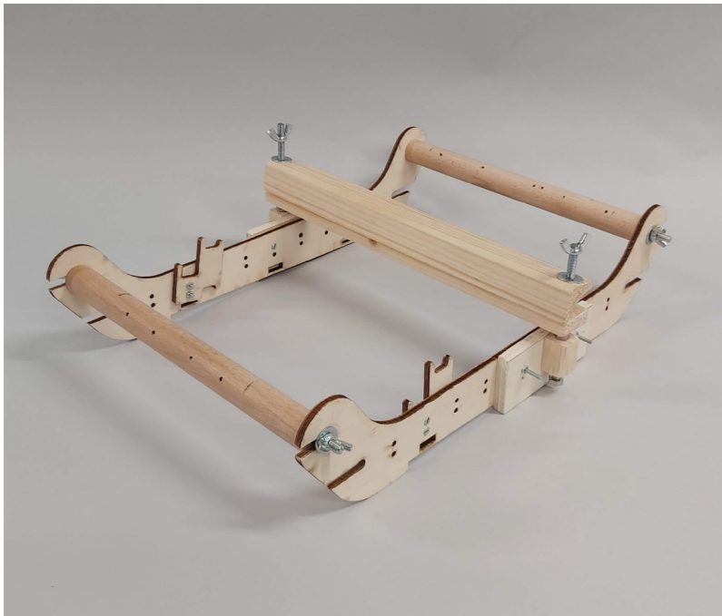
Figure 120: Prototype of the clamp on the rigid heddle loom
