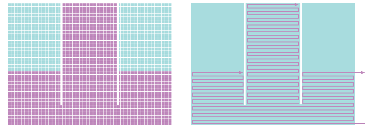
Figure 148: Visual showing how a gap in the weaving plan (left) indicated the use of separate weft threads (right)
