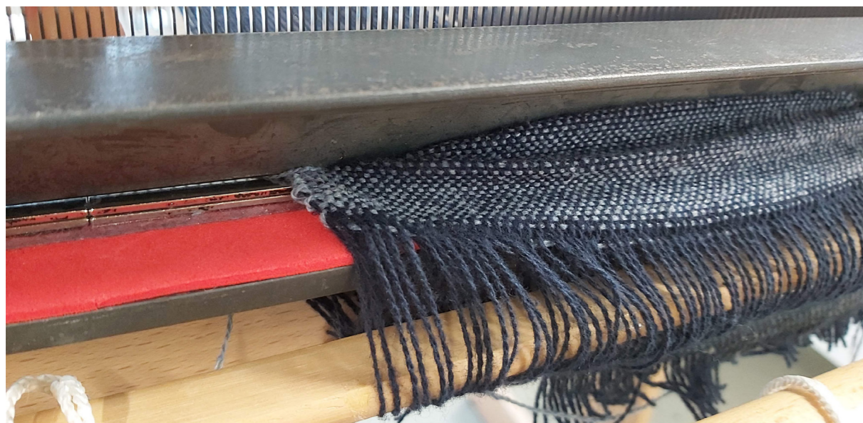
Figure 187: Picture showing the fabric bunched up against the reed and the clamp falling onto double up fabric as a result
