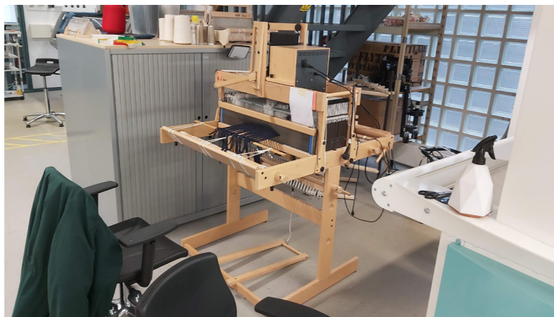
Figure 109: Louët Magic Dobby Electronic loom
