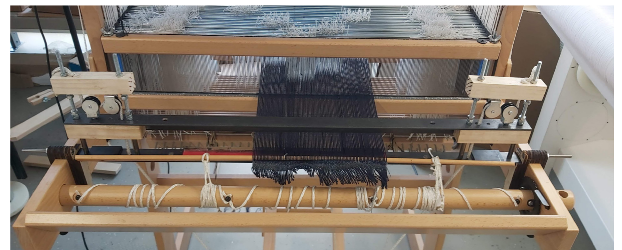
Figure 140: Picture showing how the two clamp halves are placed under and on top of the warp, which is kept in place by the rod attached to the cloth beam
