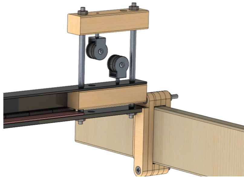
Figure 128: CAD model showing how the clamp is attached to the side of the loom
