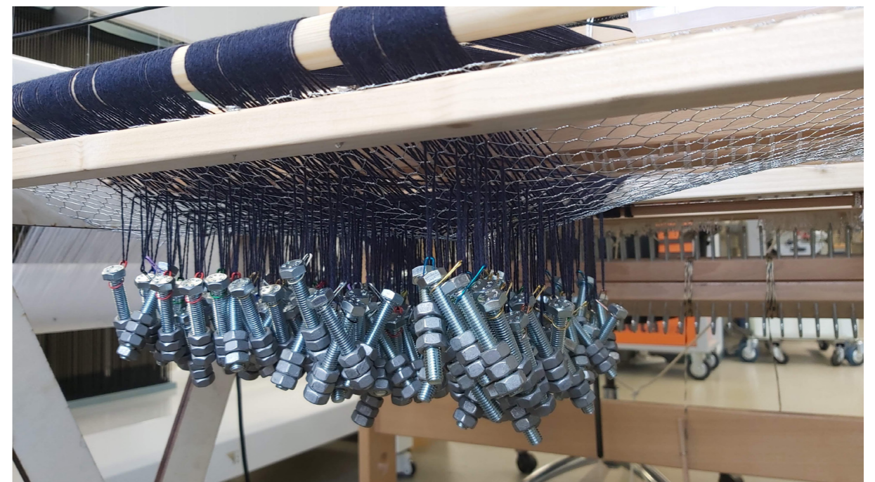
Figure 143: Setup 2 in which each individual thread is weighed down with a 30gr weight
