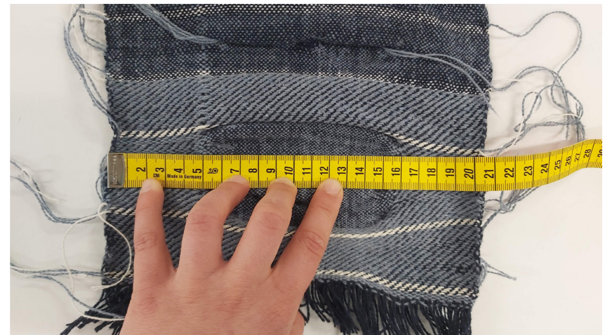
Figure 194: Picture showing how the plain weave and twill areas were measured
