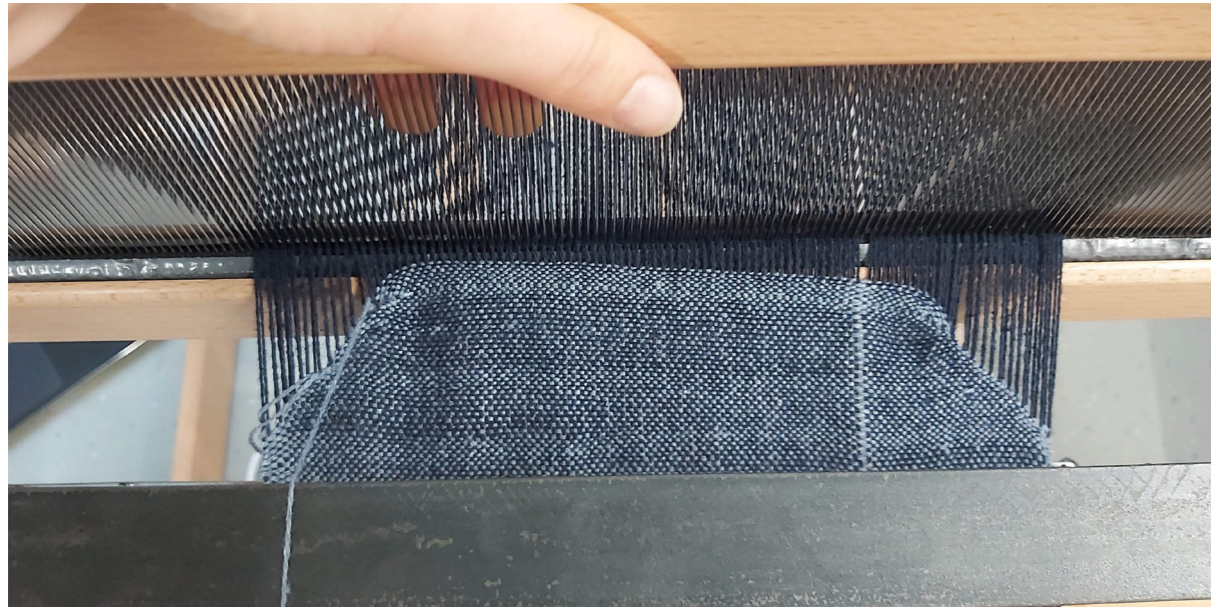
Figure 186: Picture showing a fell that has become strongly curved due to the interlacement of discontinuous weft threads
