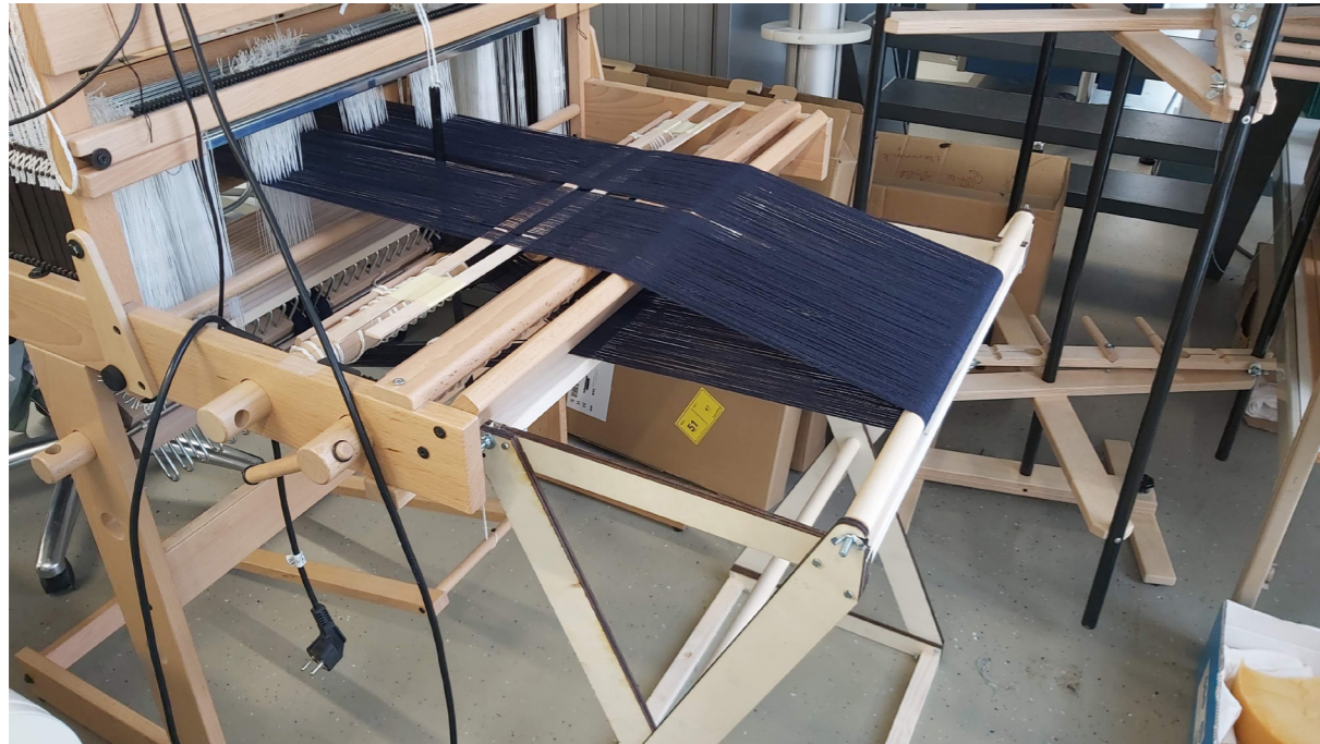
Figure 141: Picture showing how the beam of the let-off frame is inserted under warp threads, pulled back and attached to the let-off frame
