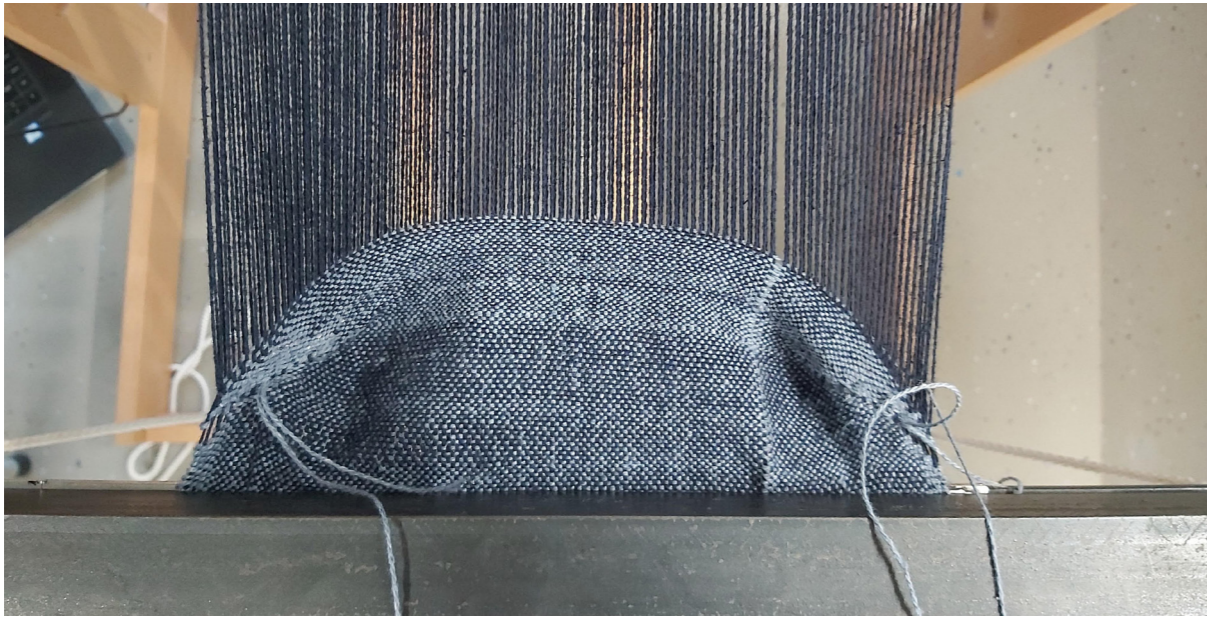
Figure 190: Picture showing how the curving weft threads pulled the warp threads in at the sides
