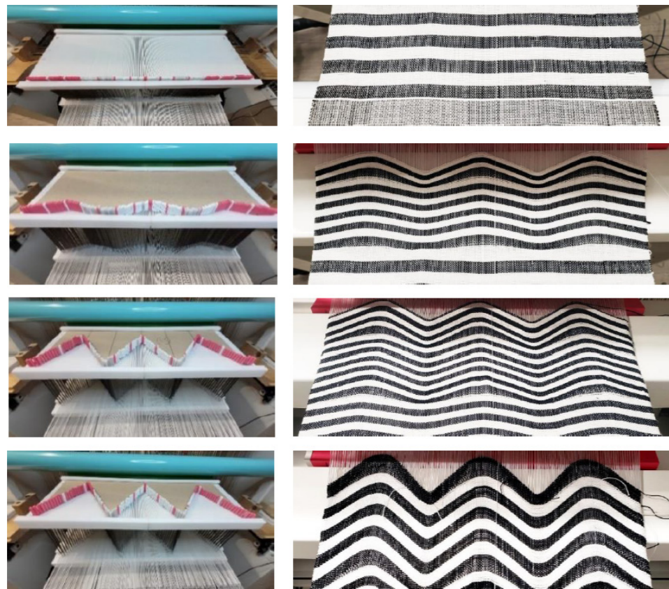
Figure 55: A variable reed of which the dent wires can be moved along the Y-axis in order to change the curve of the weft (left) and the resulting fabric while on the loom (right) (Cnaani & Sterman, 2023)
