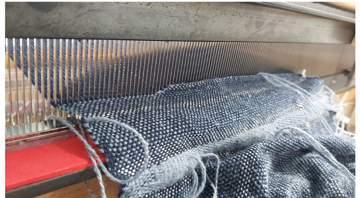
Figure 184: Picture showing how the fabric rises up against the reed
