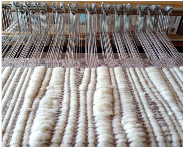
Figure 33: A rail reed in use (RailReed, n.d.)
