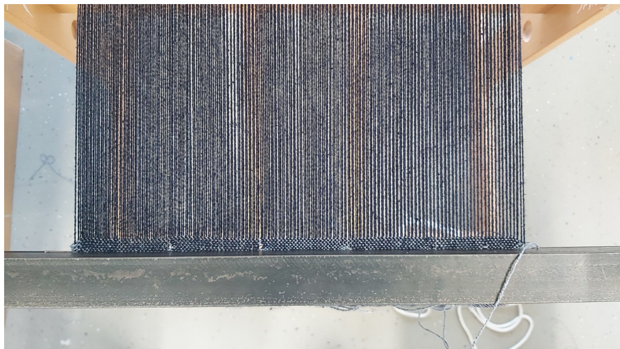
Figure 1: Picture showing how the fell remained straight as the warp threads were tensioned and a few rows of weft were woven in
