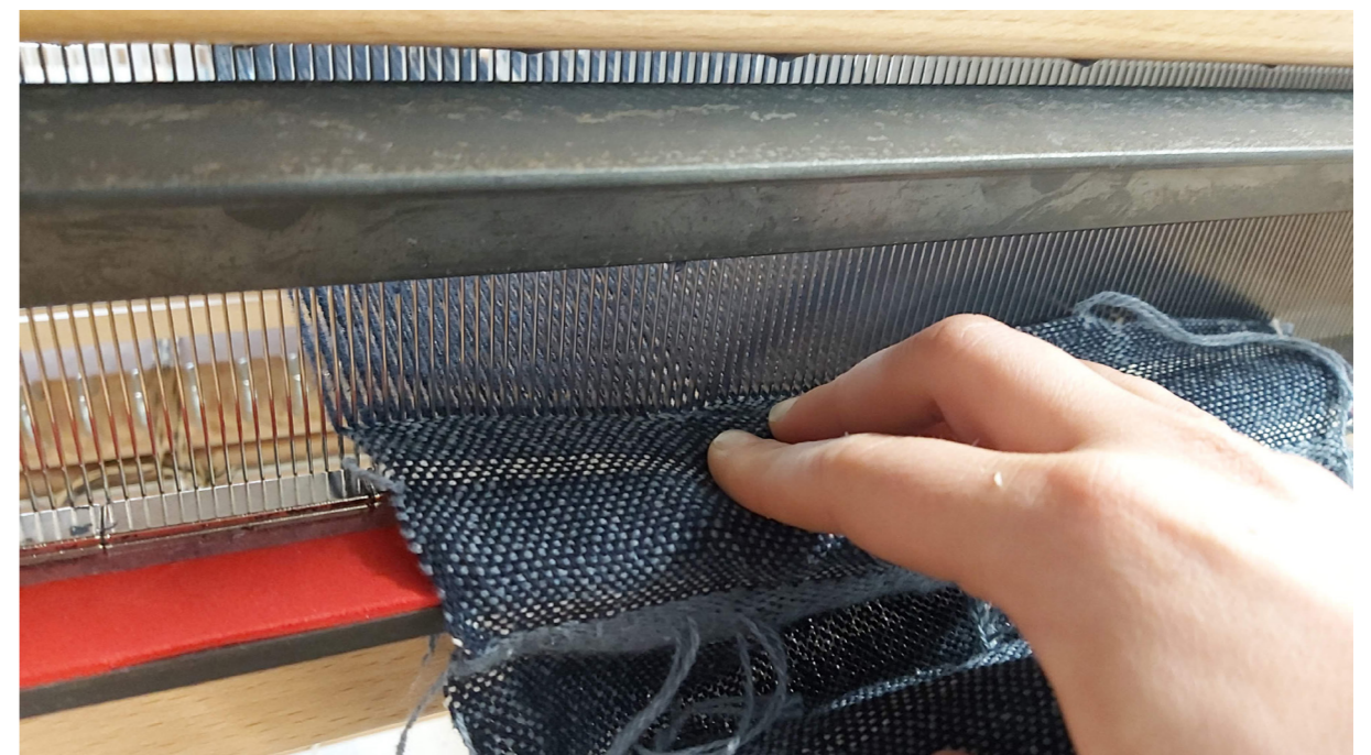
Figure 185: Picture showing how the weaver manually pushes the bulge down
