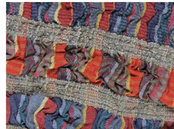
Figure 17: A double cloth made to pucker due to elastic thread being woven into one side
