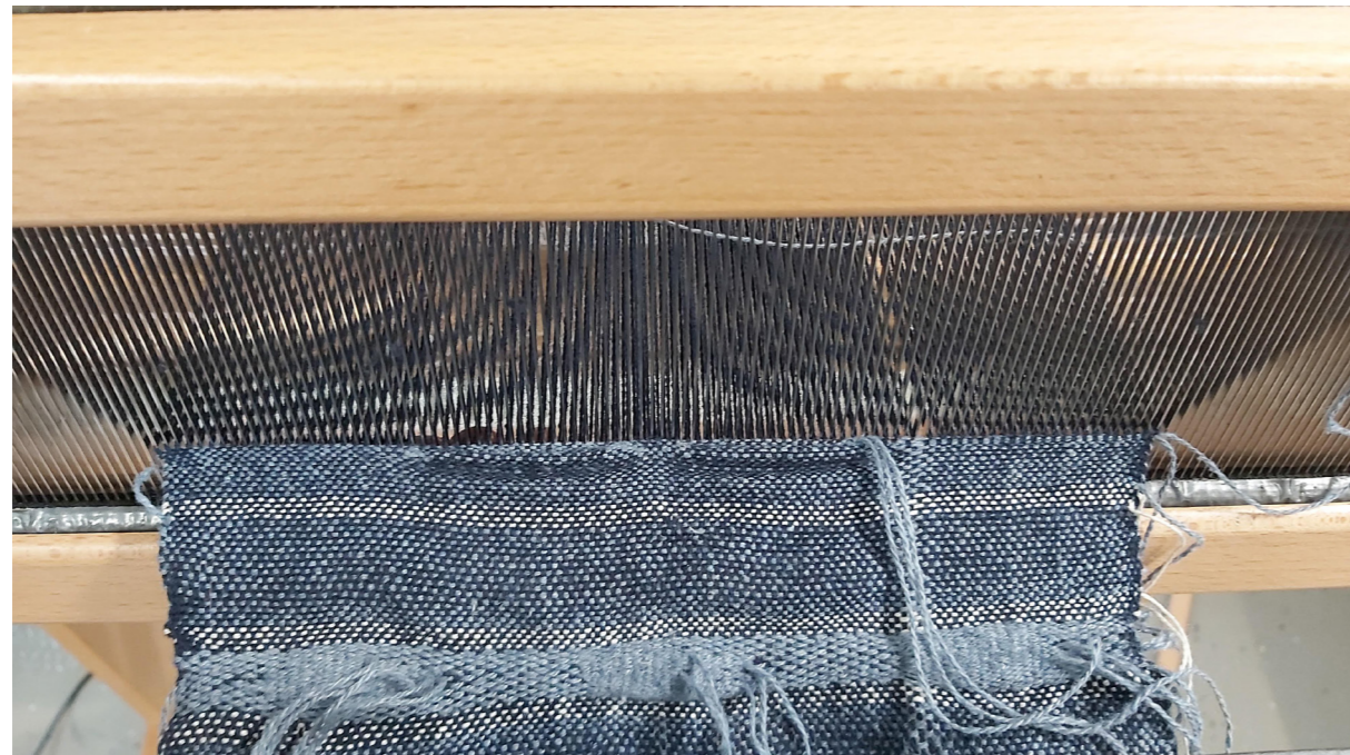
Figure 4: Picture showing how the fell is straightened by the reed
