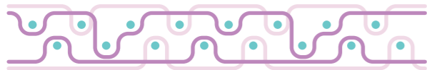
Figure 65: Illustration of a multi-layer weave structure in which the layers are connected by a common thread
