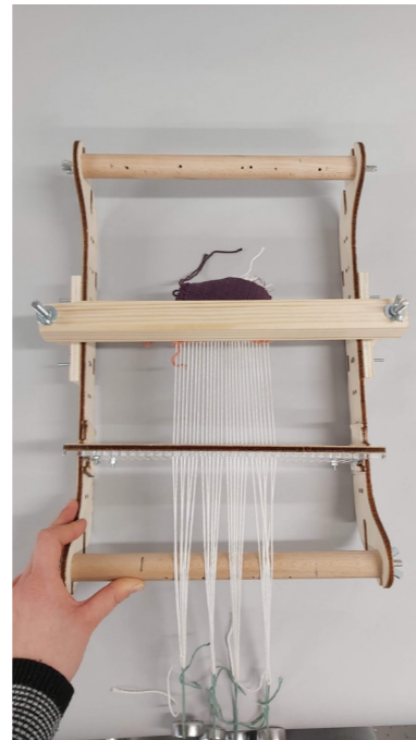
Figure 121: Loom setup with warp threads tensioned with weights
