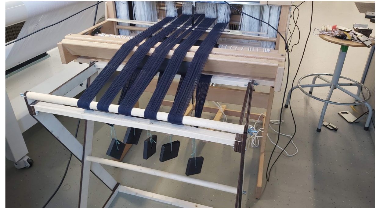
Figure 142: Setup 1 in which the warp threads are divided into five groups, each weighed down with a 500gr weight
