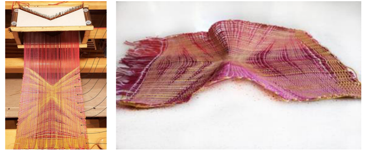
Figure 56: Example of the fabric while on the loom, showing the varying weft spacing (left), and the resulting 3D fabric that emerges when the fabric is taken off the loom (right) (Cnaani & Sterman, 2023)
