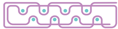
Figure 67: Illustration of a multi-layer weave structure in which the weft thread continues between the rows and the layers
