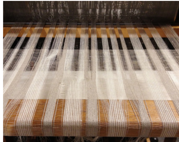
Figure 34: An open reed in use (RealFibers, n.d.)
