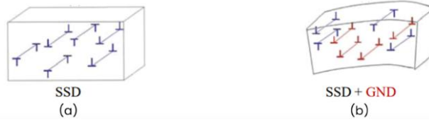
Figure 7: Effect of (a) SSD and (b) GND accumulation on crystal lattice curvature [46]
