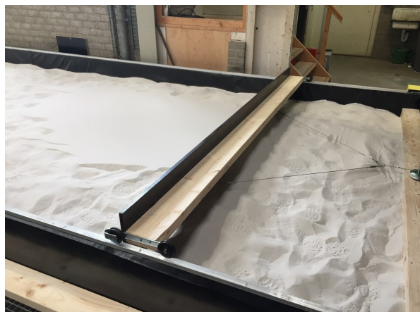
Figure 3.9: (l) Largest of the three level tools during first test and (r) sheave beam including steel sheave
