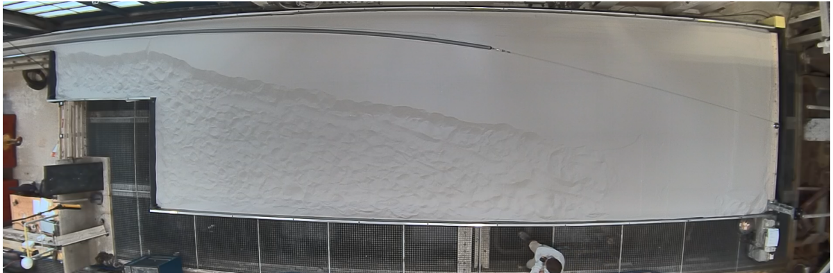
Figure 3.6: Top view of the large part of the test setup, including the sand holding flume
