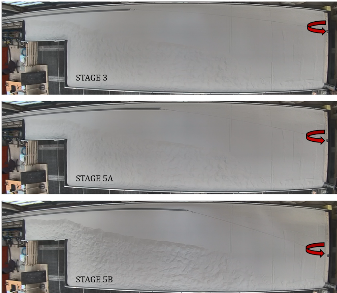
Figure 4.3: Repositioning of the sheave along a test sequence, to maintain the maximum lateral force possible on the pipe head
