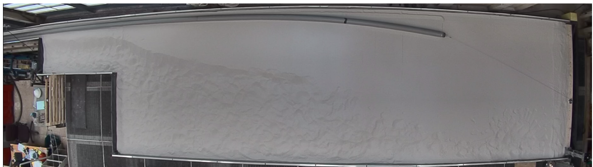
Figure 4.25: Experimental test result of the D_0 110mm ( t=3.2\text{mm} and W=8.4\text{kg/m} ) model pipeline breakout pull
