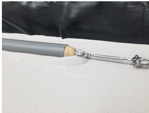
Figure 3.3: Pull head of the D_o=50\text{mm} and t=1.8\text{mm} test model during an experiment
