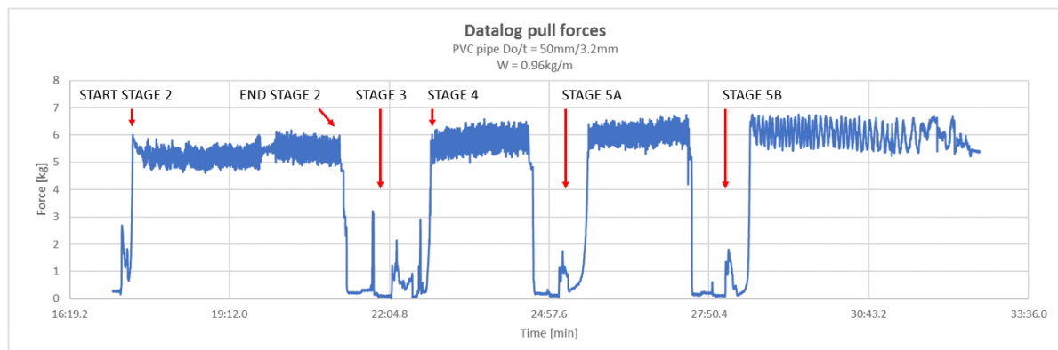
Figure 4.5: Datalog pull forces controlled pull example test
