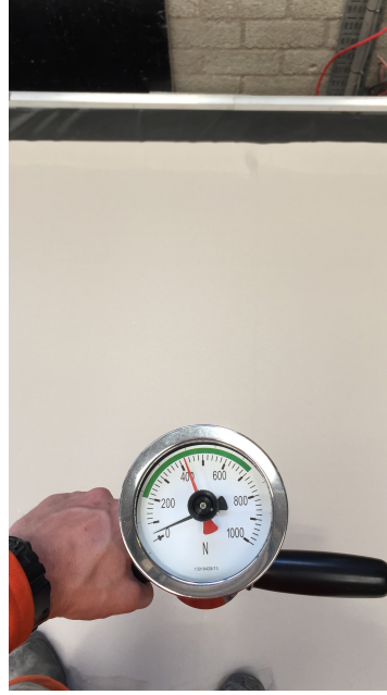
Figure 4.16: Manual CPT's to determine the sand compaction
