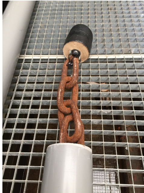
Figure 3.11: Anchor chain ballast installation of the 110 mm model test pipeline (fixed to pull head)
