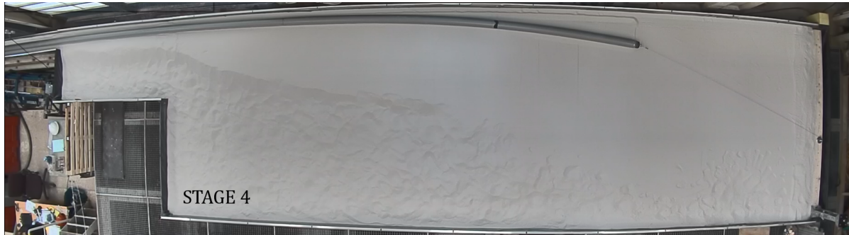
Figure 4.9: Model pipeline during a lateral breakout, showing no axial propagation
