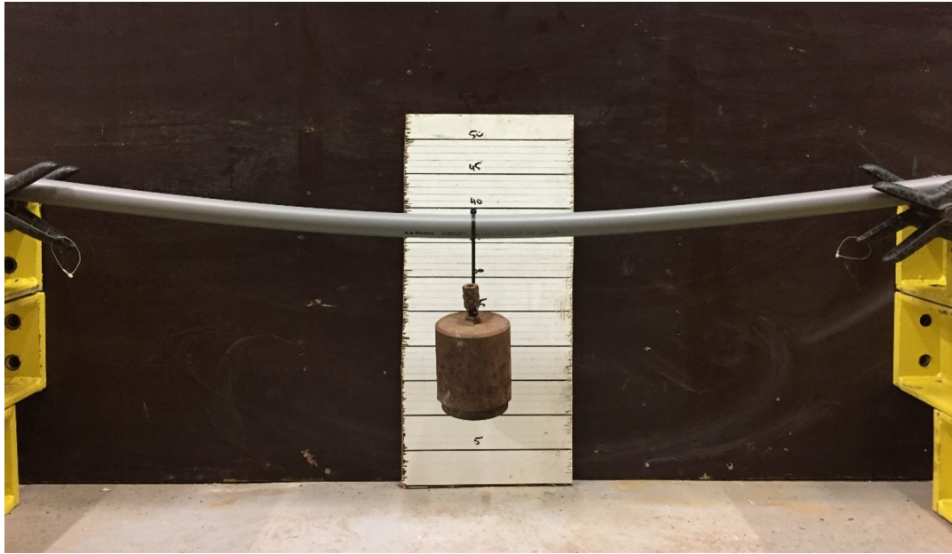
Figure 3.4: D_o=50\text{mm} and t=1.8\text{mm} test model during a bend test
