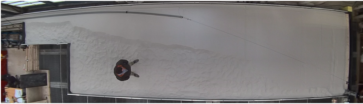
Figure 4.26: Experimental test result of the D_0 50mm ( t=3.2\text{mm} and W=1.29\text{kg/m} ) model pipeline breakout pull
