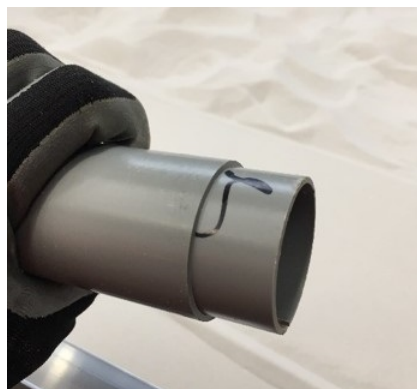
Figure 3.10: Socket connection of the 50 mm - 3.2 mm model
