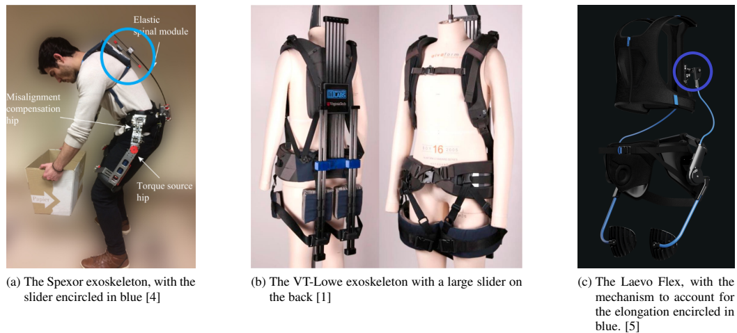
Figure 1.1: Three examples of current exoskeletons with sliders or some other mechanism (Laevo)
