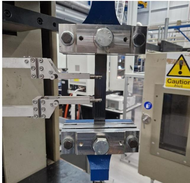
Figure 61. IPSS test setup
