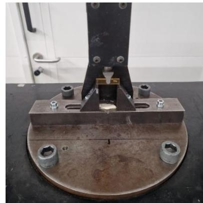
Figure 48. SENB sample installed in the fixture
