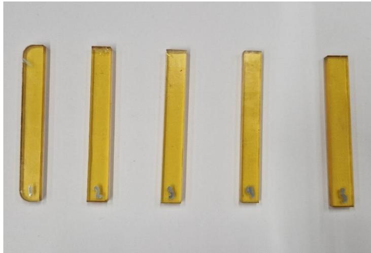
Figure 43. RTE specimens for 3PB
