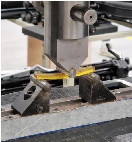
Figure 42. RTE sample loaded in 3-point bending
