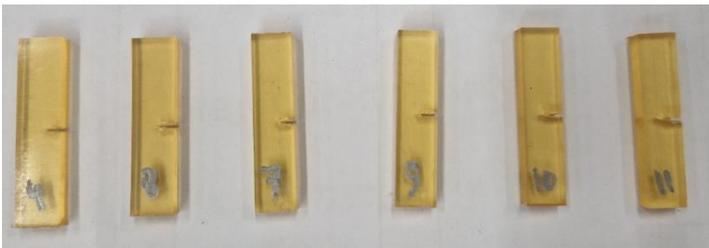
Figure 47. RTE-DDS SENB specimens
