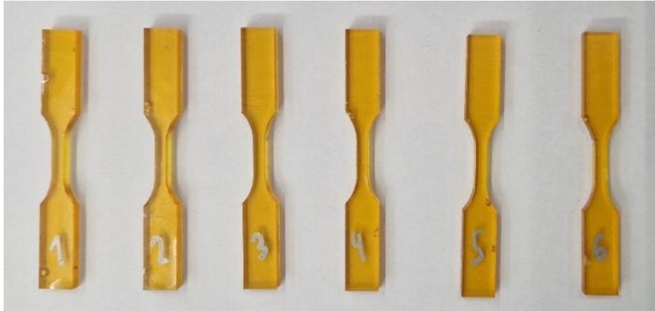
Figure 39. RTE-DDS tensile samples
