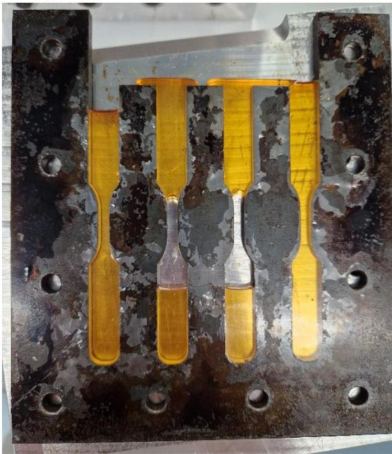
Figure 37. Tensile mould not filled in due to trapped air
