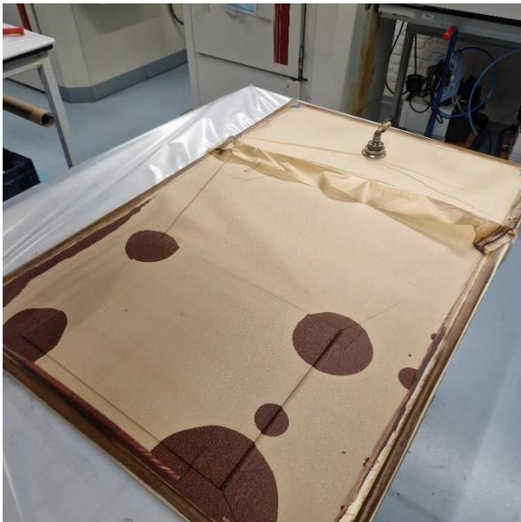
Figure 53. Vacuum bag after curing
