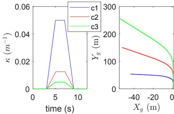
Fig. 3: The tested curves c1, c2 and c3, shown in birds eye-view as a function of global  $X_g$  and  $Y_g$  coordinates, and the corresponding curvature profiles  $\kappa$ .
