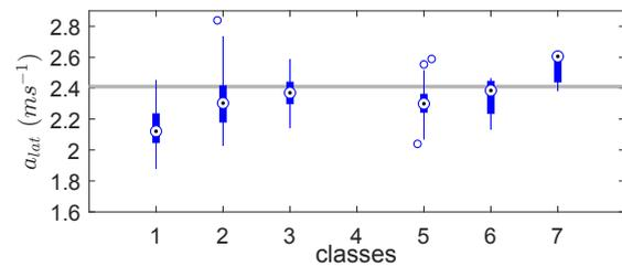
Fig. 7: The differences in average  $a_{lat}$  in the curve, given for all curves driven. A line at  $2.41 \text{ m/s}^2$  is outlined to represent  $a_{lat}$  when the centerline of the curve would be followed.
