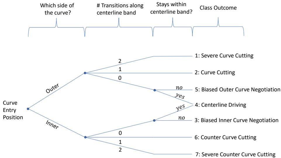
Fig. 2: A decision tree illustrating the rule-based classifier deduced from knowledge of the driver trajectories found in this paper. The centerline band is taken at  $\pm 0.1$ m from centerline.
