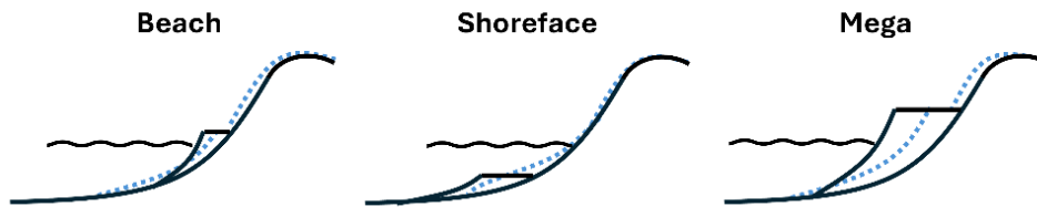
Figure 1.2 Schematic cross-shore representation of beach, shoreface, and mega-nourishment types. Blue dashed lines indicate the post-placement equilibration process, where nourished sand redistributes toward a more natural beach profile under wave and current forcing.
