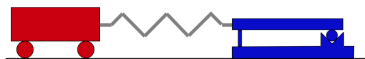
Fig. 2: Schematic overview of the position-controlled actuation system setup with the linear guide (red), spring (gray), and actuation system with end stop (blue).
