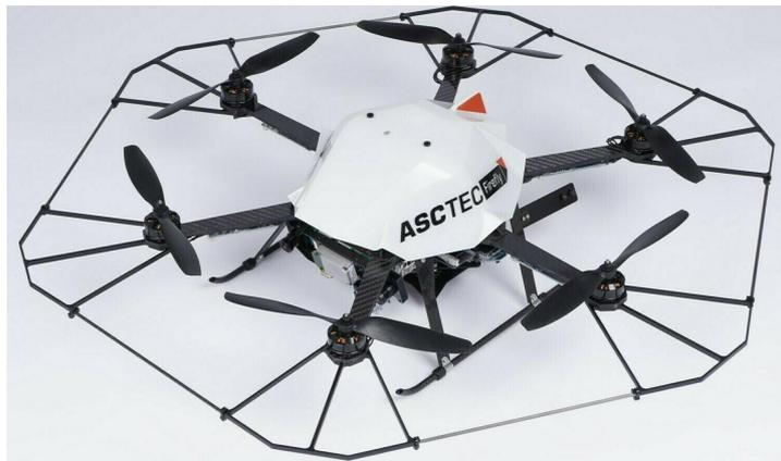
**Figure 2.4:** AscTec Firefly hexacopter, which the default coefficients are based on (<https://productz.com/en/asctec-firefly/p/w9DR>).
