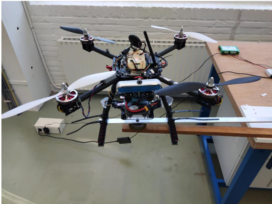
**Figure A.5:** Torque setup quadcopter leg supports.
