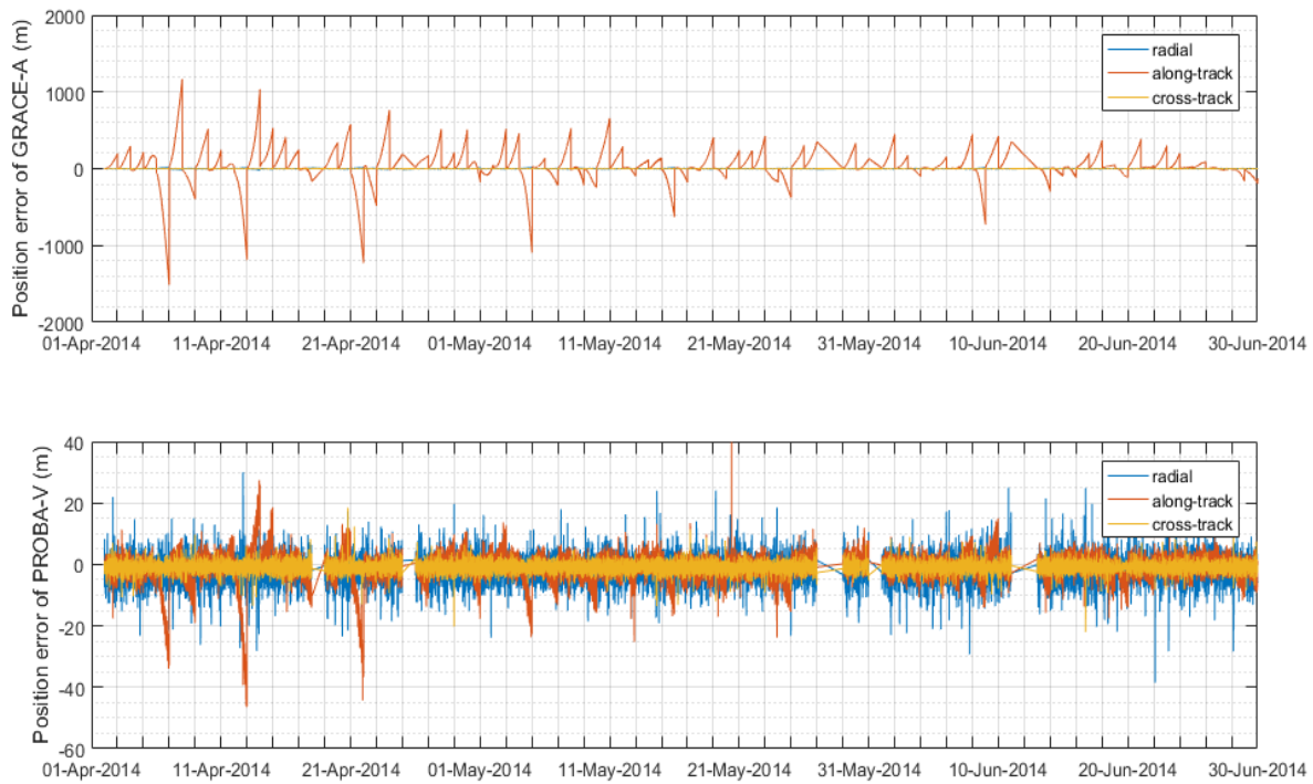
(a) Position errors of GRACE-A (top) and PROBA-V (bottom) resulting from orbit prediction using C_d of previous day, during April - June, 2014 - best prediction method.
