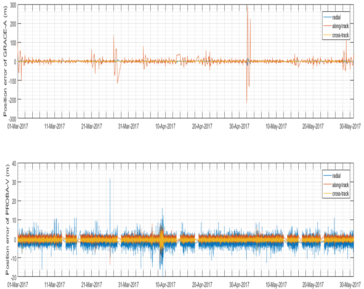
(a) Orbit estimation ( 1 C_d per day) position errors for GRACE-A (top) and PROBA-V (bottom) during March - May, 2017.
