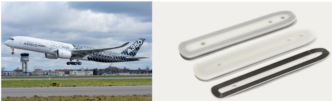
Figure 1: On the left the Airbus A350 for which main components are constructed from carbon fibre reinforced material (source: Airbus). On the right 3D printed examples reinforced with carbon fibres in the contour (source: MarkForged)
