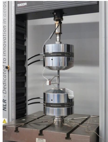
Figure 8: Results of the tensile tests for five coupons and test setup on the right
