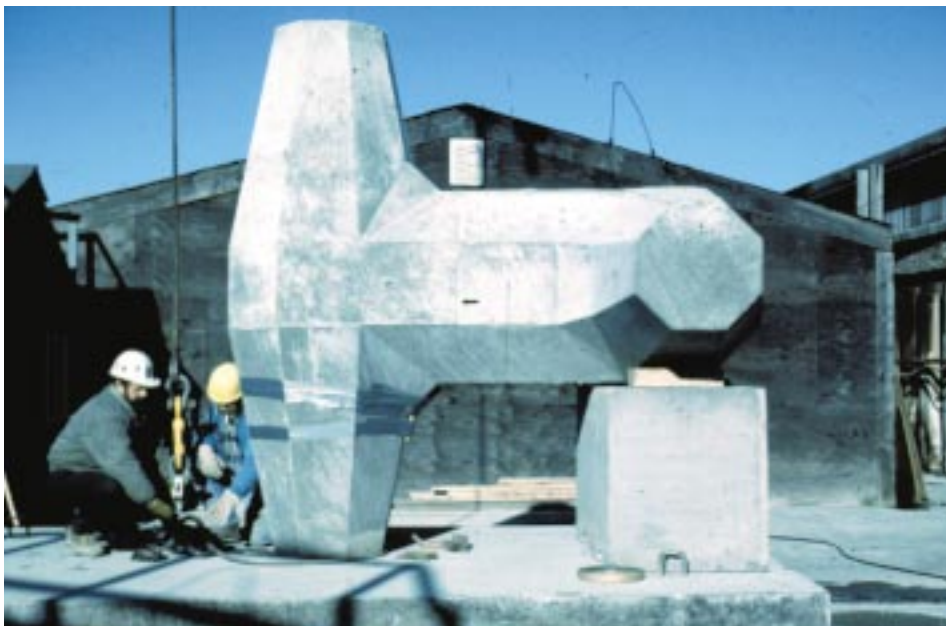
Figure 2. Standard dolos drop test
