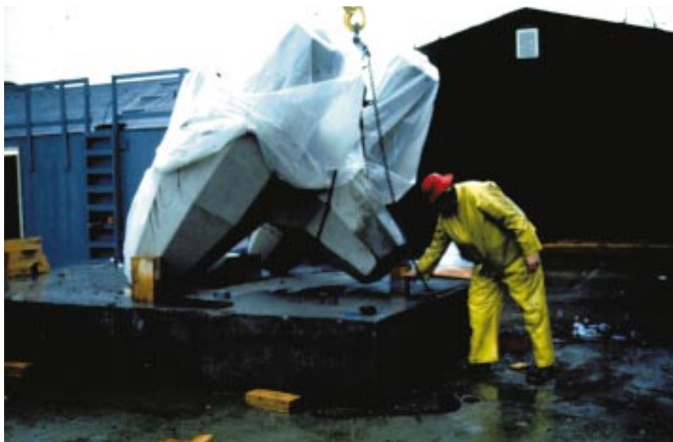
Figure 1. First Core-Loc drop test
