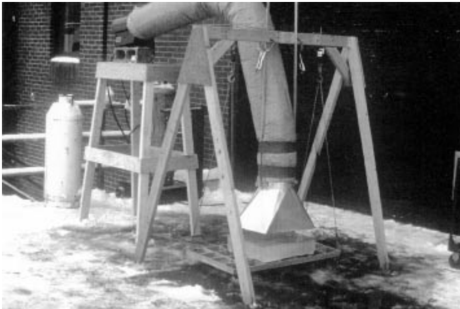
Figure 1. Setup for space heater tests
