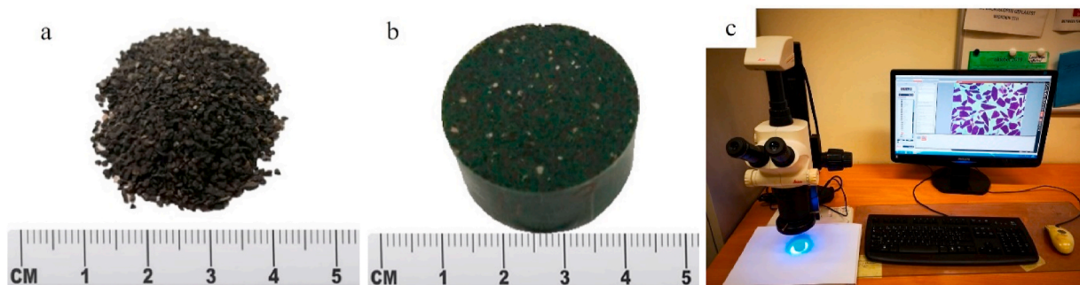
Fig. 3. Sand particles (a) and sample for image acquisition (b) under optical microscope (c).
