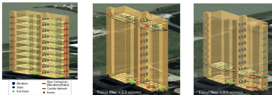
Figure 24: 2D floor plans embedded in 3D space and linked to the outside network (Thill, et al 2011).
