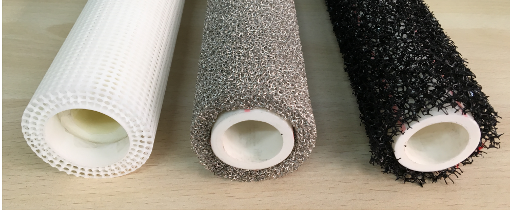
Fig. 1 Examples of porous coated cylinder types, illustrating the differences in porous coating structures that are used to treat cylinders as a form of passive noise control (from left to right: SPCC, MFPC and PPCC).
