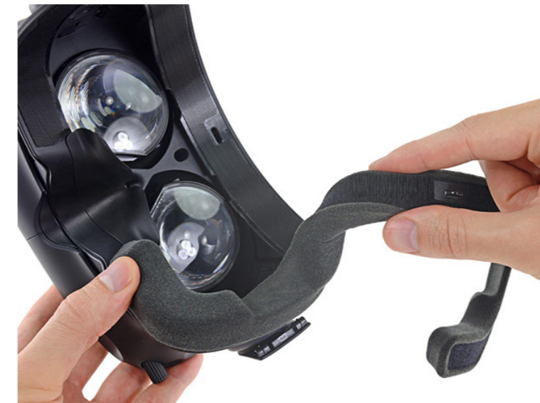
Velcro attachment system (www.vive.com)
