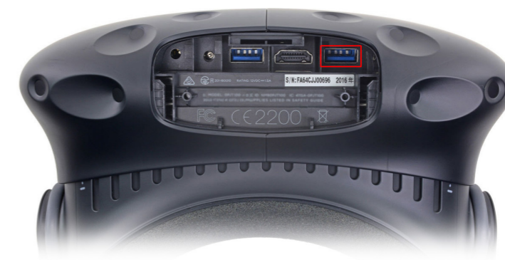
Top view of uncovered HTC Vive showing the connection ports (www.vive.com)
