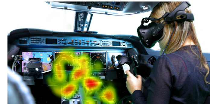
Simulation of an aircraft in VR integrated with eye-tracking data (www.tobii.com)
