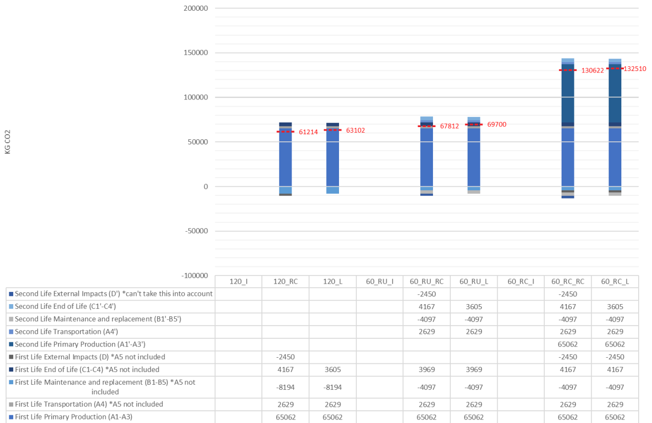
Figure 53: Standard Concrete (including the carbonation during lifetime)
