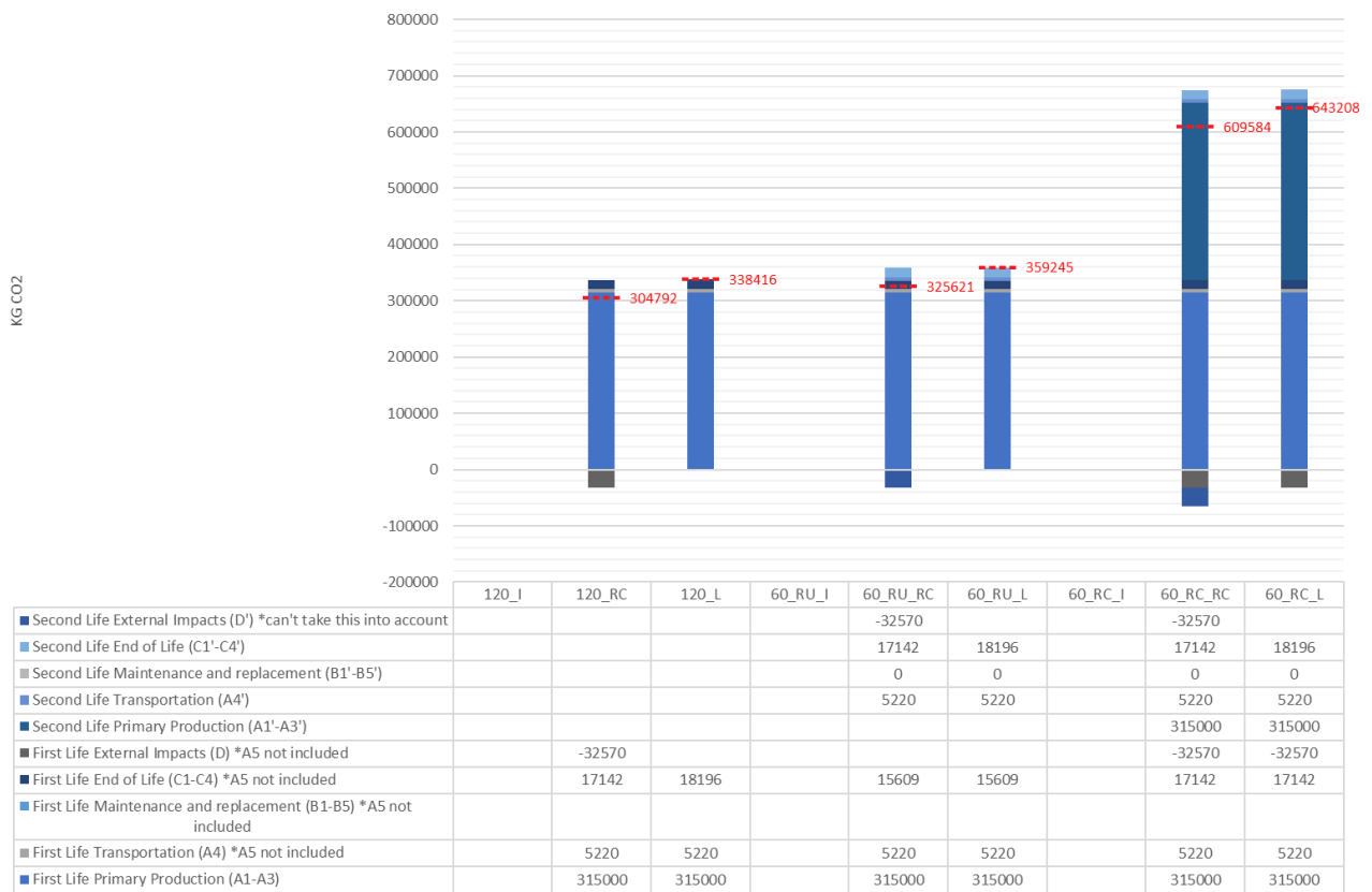
Figure 63: Standard Concrete (including the carbonation during lifetime)
