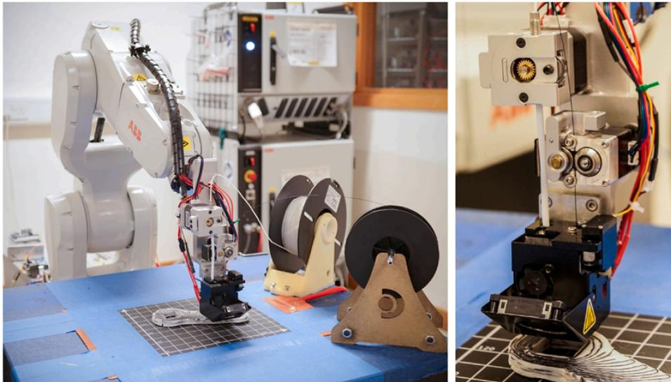
**Fig. 11.** The hardware setup for fabricating specimens used in our physical experiment to test the mechanical properties when different toolpaths are applied.
