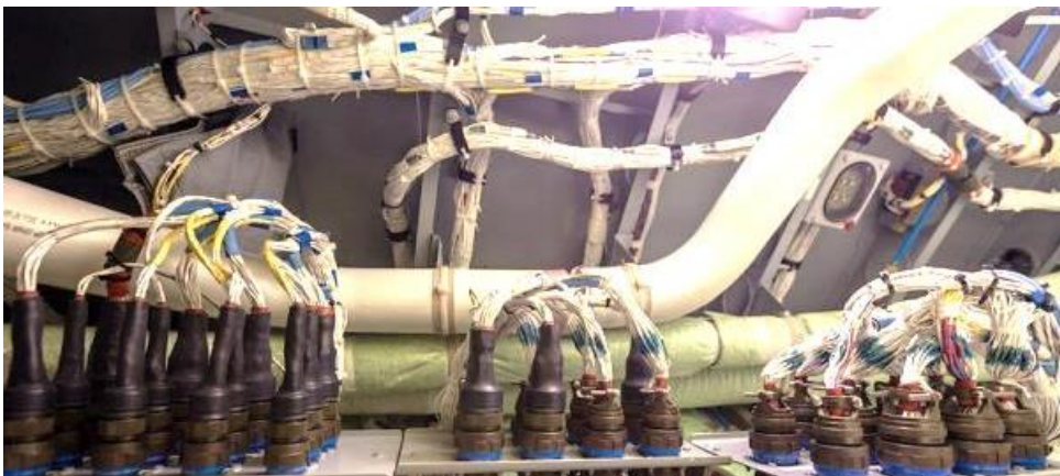
Figure 1-2: Wire harnesses in the Russian Sukhoi Superjet 100 [5]
