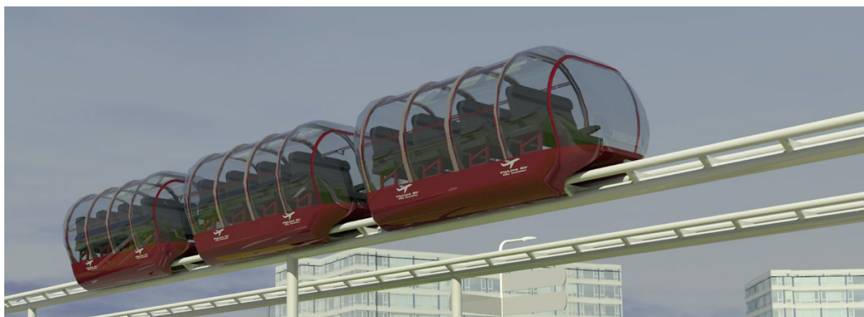
Figure 1-1: The City Coaster, three automated vehicles on a roller coaster track
