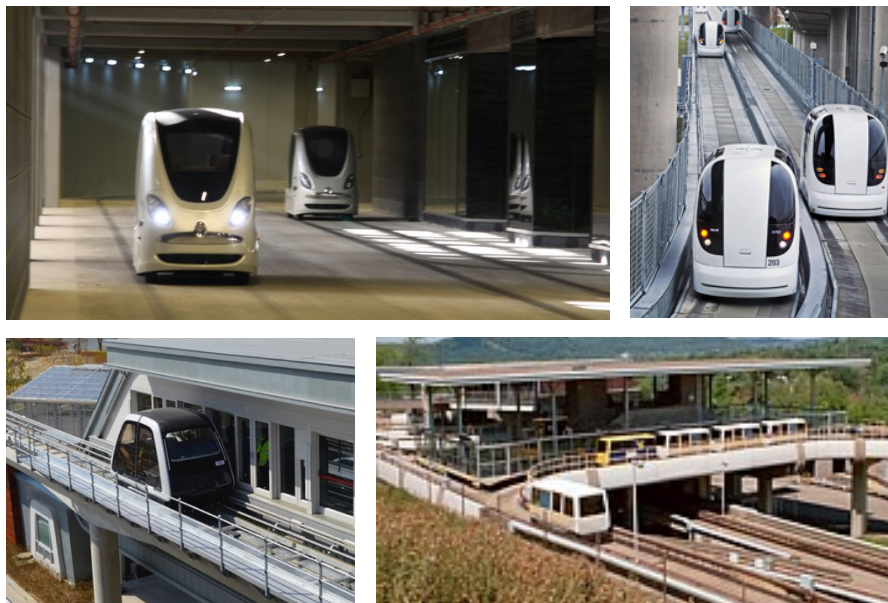
Figure 2-2: Upper left: Masdar PRT, upper right, London Heathrow, lower left (Suncheon PRT) lower right: Morgantown PRT (reprinted from Khammas, 2017; PRT Consulting, 2015; ARUP, 2017)
