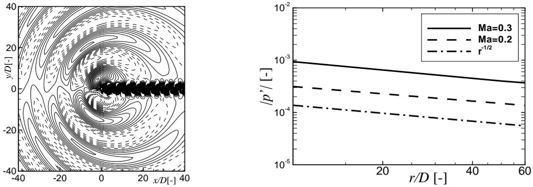
**Figure 1.** (left) Isolines of pressure fluctuations  $p'$  around the cylinder (solid line indicates positive values, dashed ones negative), and (right) decay of pressure peaks with distance  $r$  compared to the theoretical decay of  $r^{1/2}$  for two Mach numbers.
