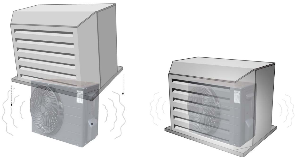
▲ Figure 5 - Placing the Brockx over an AC unit to reduce the noise of the AC
