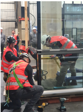
(k) Workers trying to take out the glazing, which took some force
