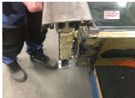
(b) Picture destructive testing, the aluminium framing, bronze cover profile and the glazing unit can be seen (Boosting, 2022)
