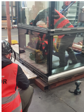
(j) The machine connected to the glazing, Cracks are forming
