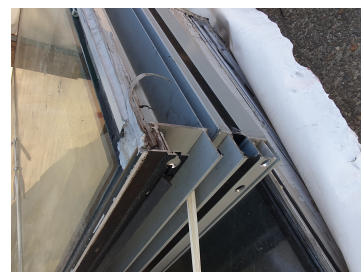
(c) The remaining cut profiles, Sealant is clearly visible
