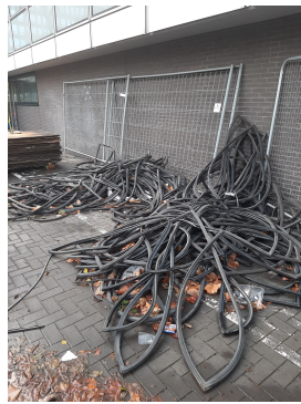
(a) Scrapped EPDM gaskets of the koningskade, made by Scheldebouw (2020)
