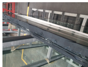
(b) The leftover sealant on the slightly damaged glazing which was cut from the aluminium framing
