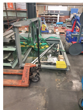
(d) The last piece of the test element, which was a corner element was taken out in one piece. Some damages can be found on the aluminium as well as some misshaping of the parts. The glazing was kept intact.
