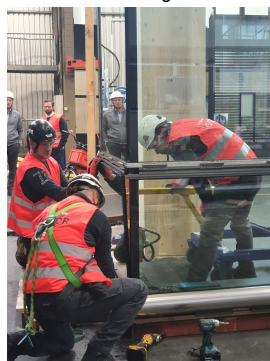
(e) Workers forcefully taking out the glazing
