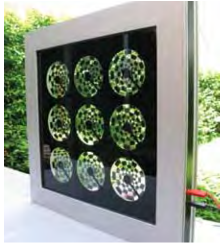
Figure 7.22: Mock-up installed in window element – motors turned off
