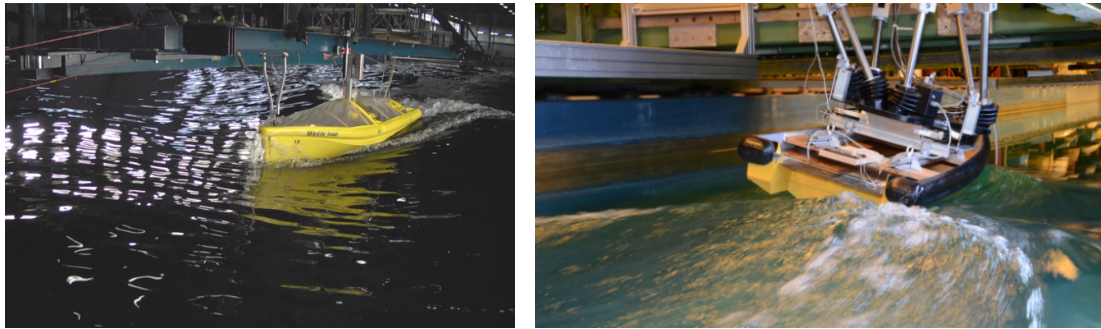
Figure 6 Model test. On the left, the set-up lets the model free in heave and pitch; on the right, the model is fully captive.
