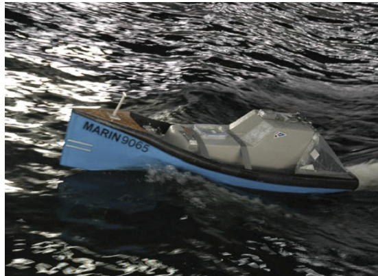
Figure 5 Free sailing model tests on an auto-propelled vessel.
