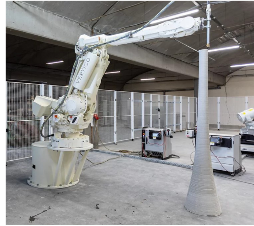
6-Axis Industrial Robot w/ Industrial Printing Head
