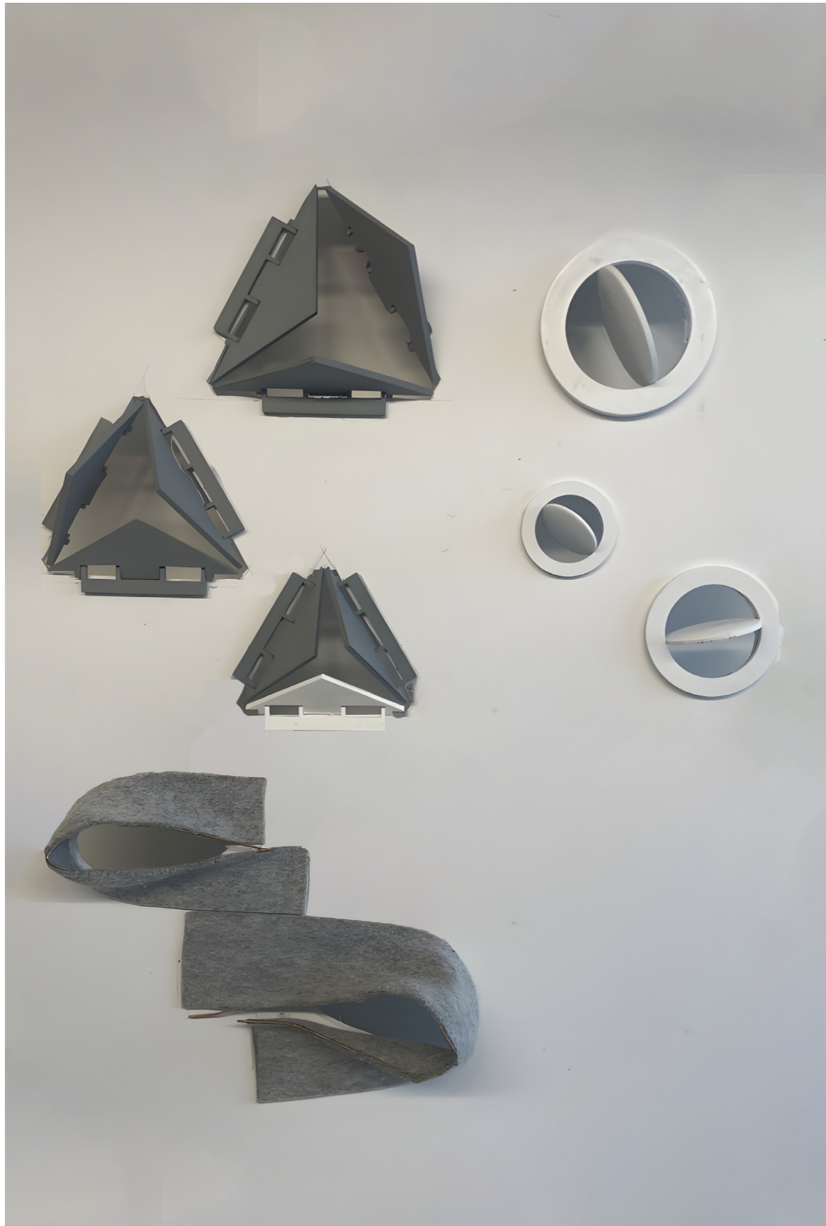
Figure 42: Ergonomic test setup of ventilation opening with hinge point in, on, and outside the plane in various sizes
