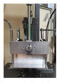
Figure 7.8: Method for measuring the relative displacement of glass and steel
