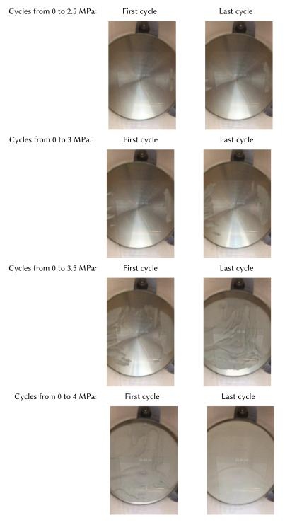
Figure 5.16: Whitening effect propagation under loading cycles
