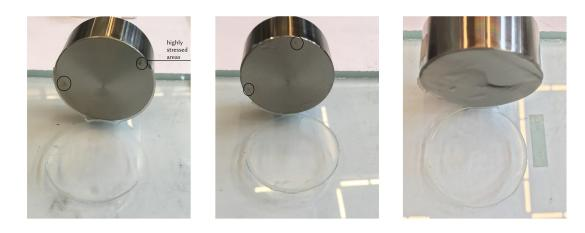
Figure 5.8: Pictures of tested specimens under monotonic loading after failure
