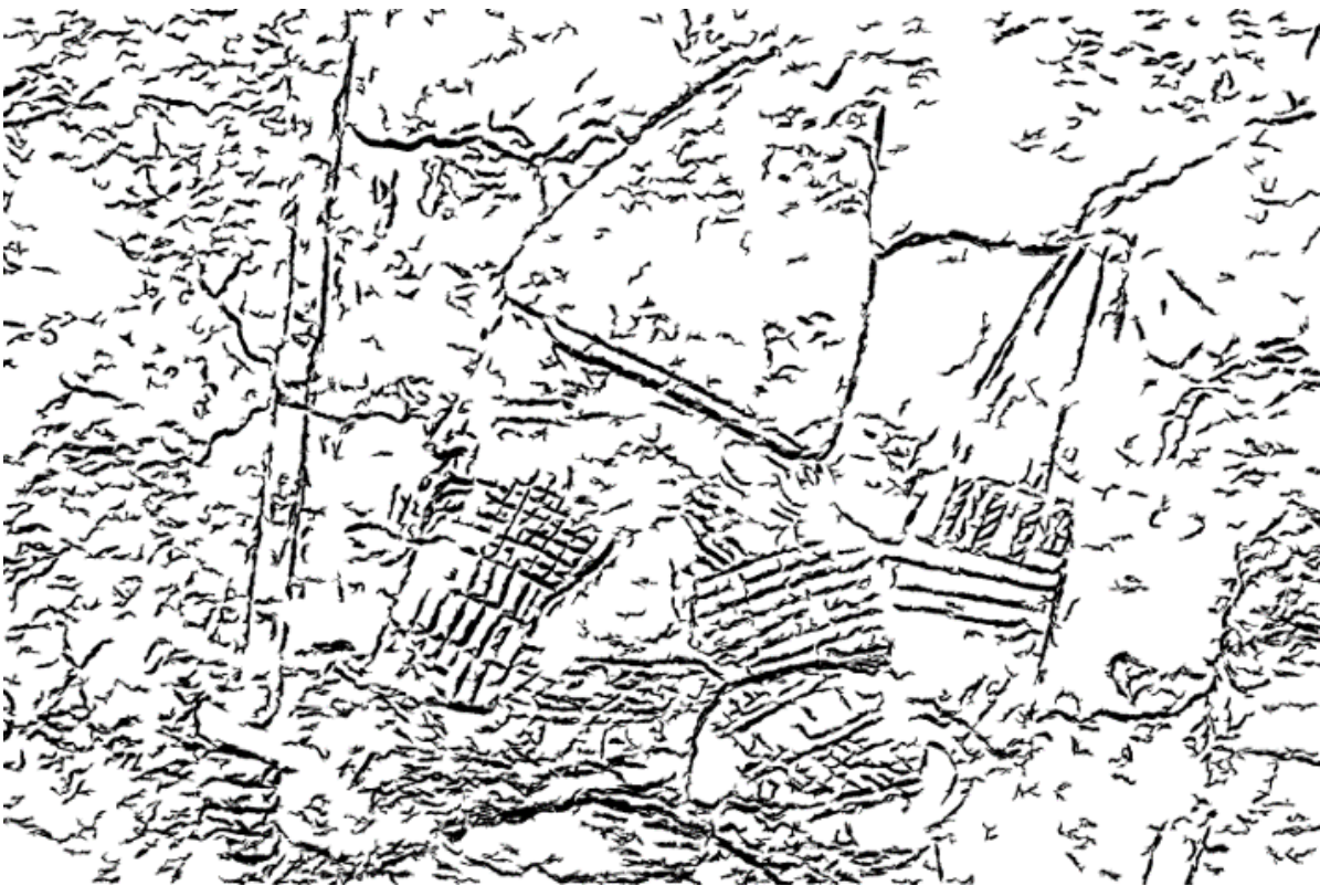
Figure B.9: Photo V34-9 filtered with SVM, which is trained with surf features. The feature length was set for 64. After filtering blobs with a size smaller than 350 pixels were removed.
