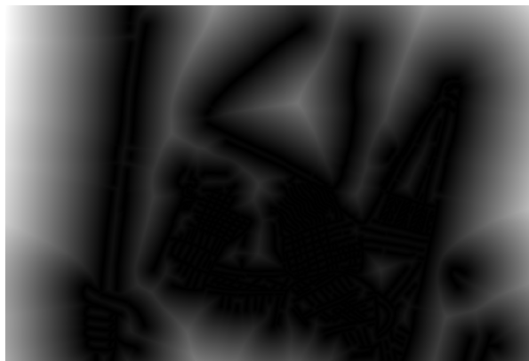
(a) The Euclidean distance of every pixels to the closest line in V34-9. Black is the lowest value and white the largest.
