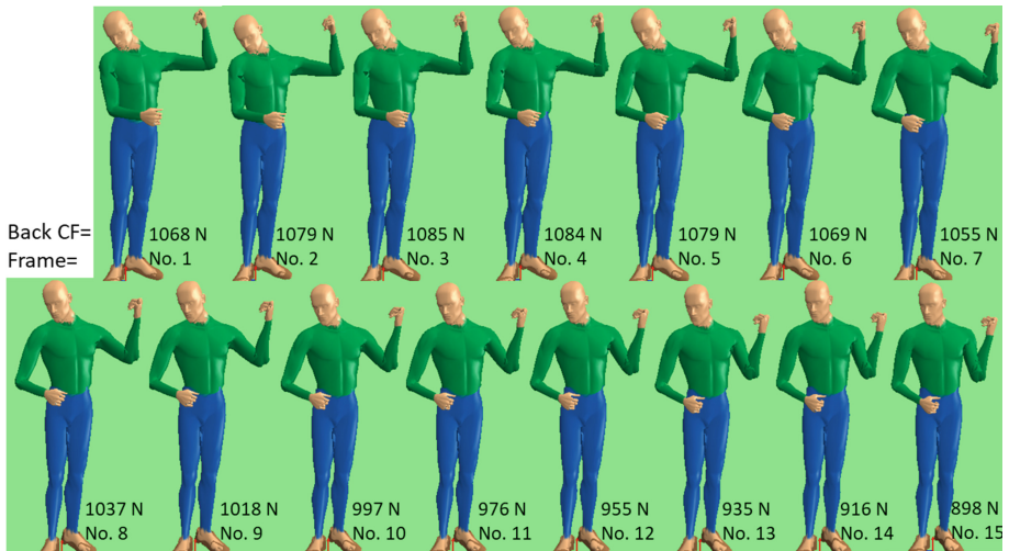
Fig. 2. A frame-by-frame distribution of Back Compression Force (BCF) in sweeping activity
