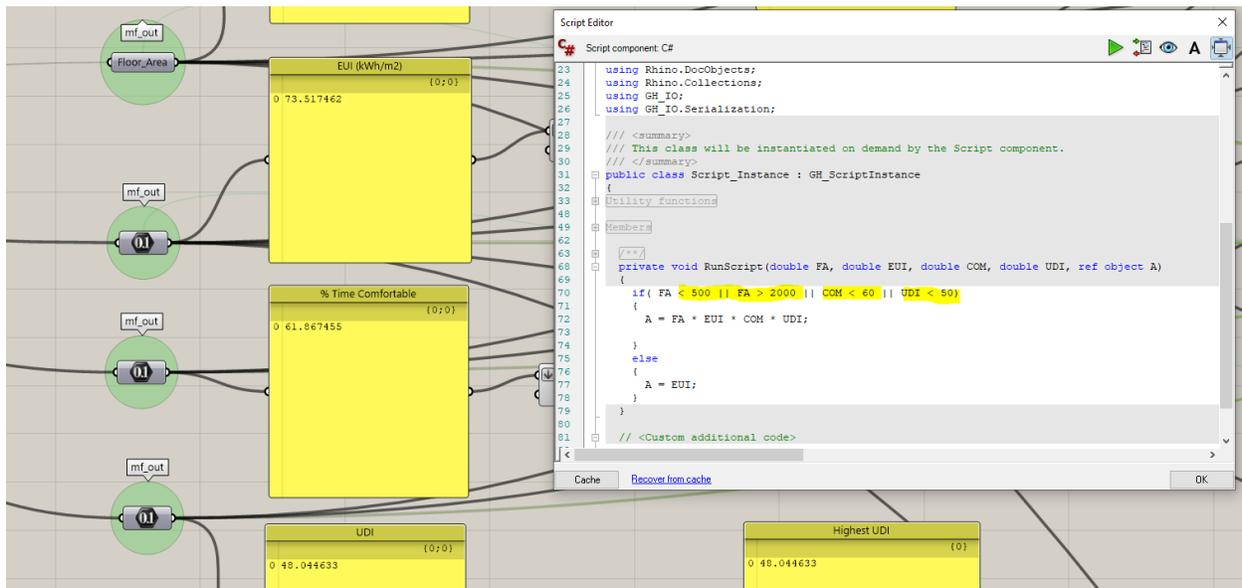
Figure 40 C# component for single Objective optimization (source: own)
