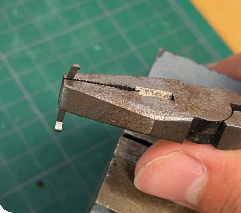
Fig. 105: Bending plasma-cut springs by hand...
