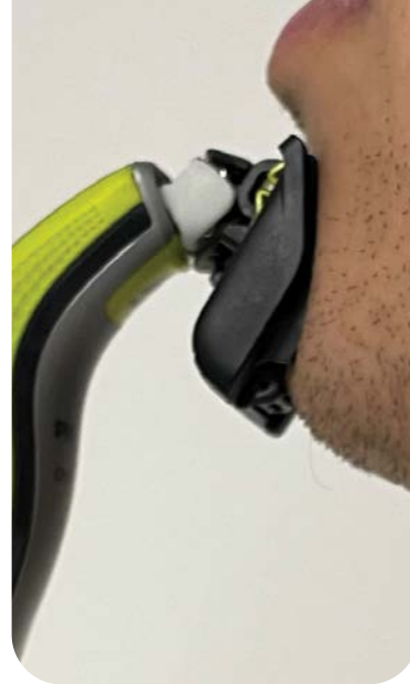
Fig. 108: Applying minimal pressure (5 in 1 comb) -> detaches
