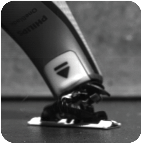
Fig. 60: 90cm hinge opens as intended
