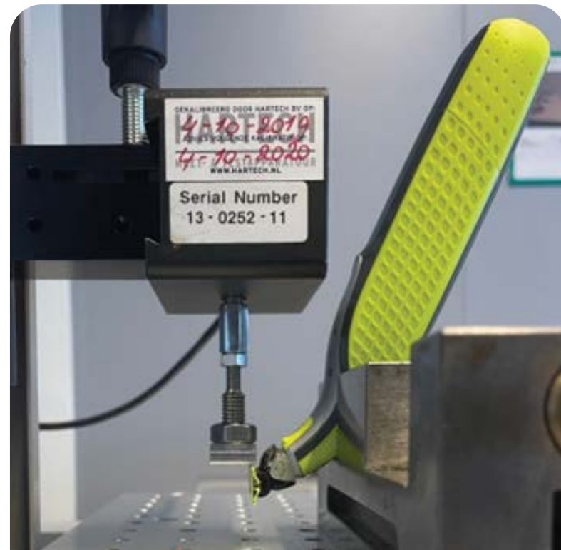
Fig. 109: Test precisely measuring force needed to detach concept V2
