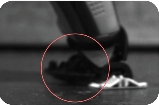
Fig. 64: 110cm hinge snap-fit breaks
