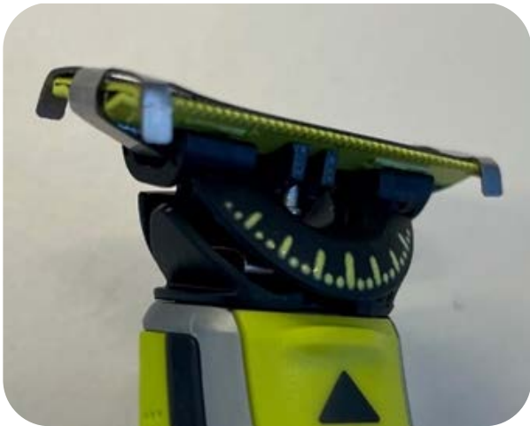
Fig. 79: MVP of the pinch-release hinge concept: Click-in snap fits are filed of, with the blade being kept in place by metal fins instead. This mimics the concept
