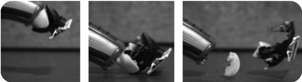
Fig. 103: 90 cm drop on the front -> 3D print breaks, giving inconclusive answers
