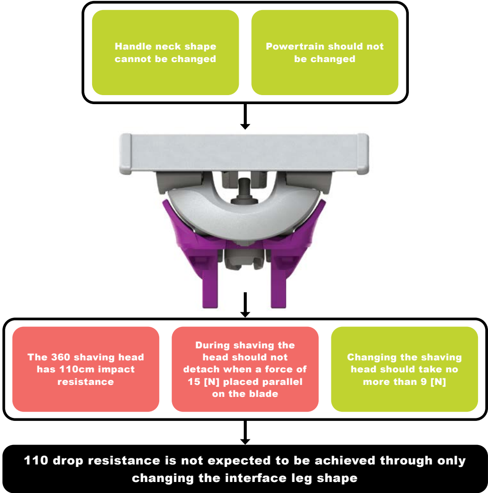
Fig. 117: Results of the validation of concept V3 and next steps
