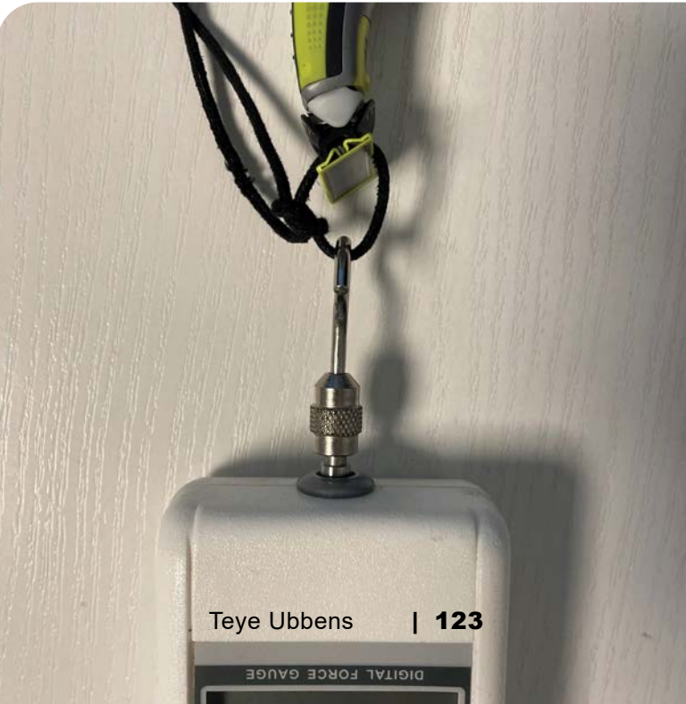
Fig. 106: ...and testing their clamping force using a force meter
