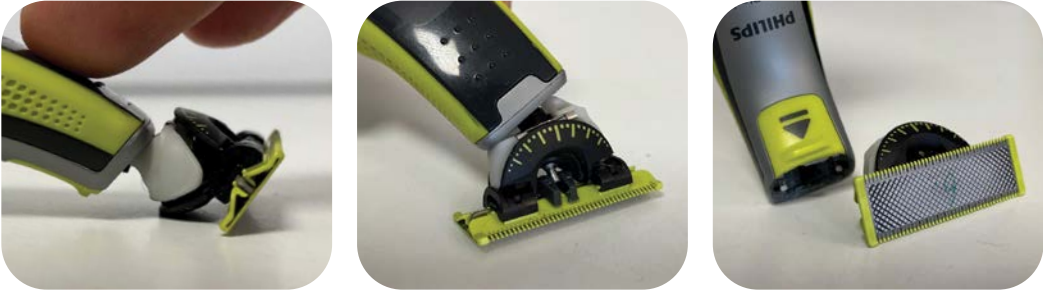
Fig. 102: 70 cm drop on top-side -> Breaks, as after the head detached the handle pushed on the font of the legs, over-rotating the hinge and breaking the front left blade snap-fits.
