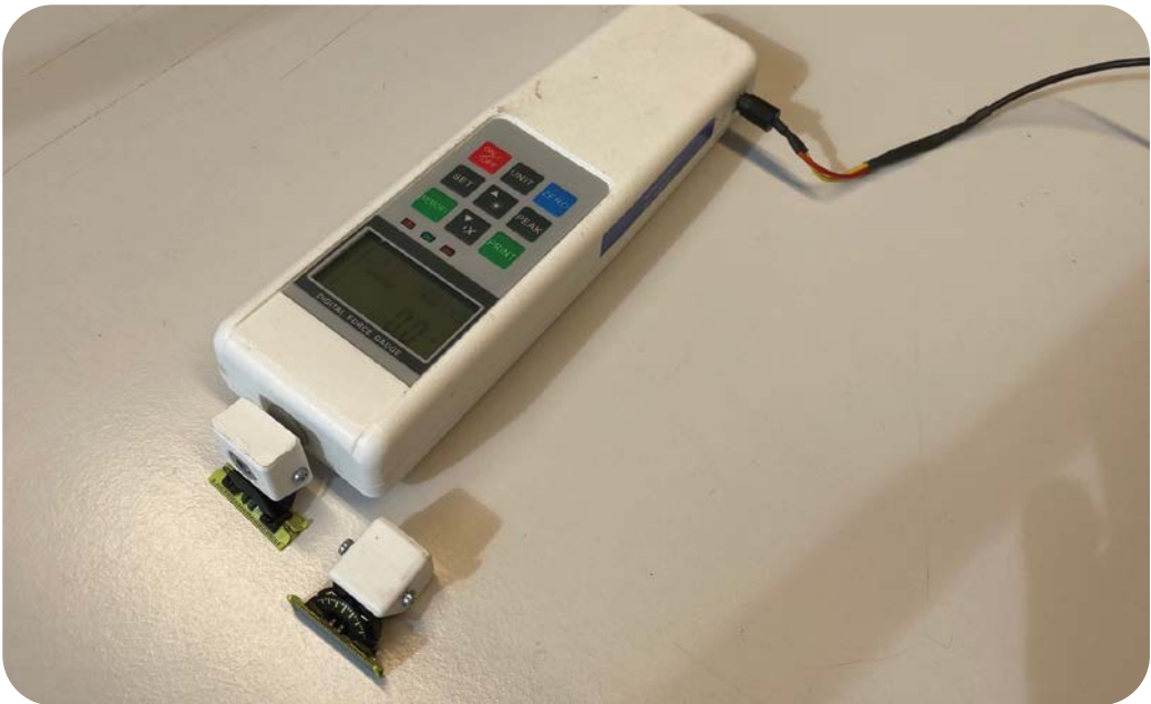
Fig. 50: The apparatus used: an MRC DFG500 digital push gauge with two 3D printed shaving heads for measuring the x and y components of shaving force.
