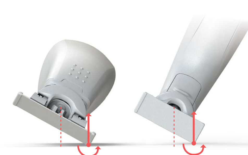
Fig. 71: Moment around side of the blade cannot be dissipated
