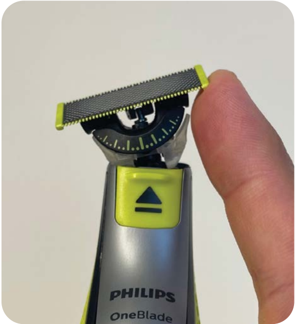
Fig. 93: Detaches with a sideways moment
