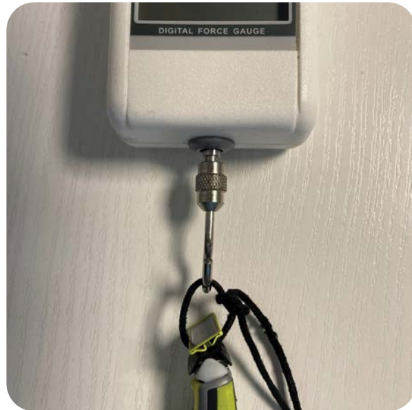
Fig. 88: Measuring force needed for detaching V1
