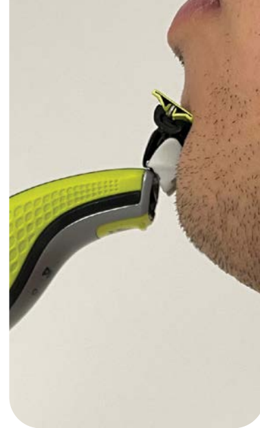
Fig. 107: Applying moderate pressure (no add-on) -> detaches
