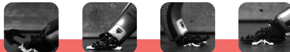
Fig. 4: Results form droptests and analyzing highspped camera footage
