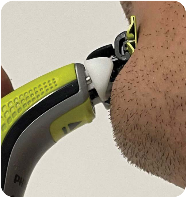
Fig. 87: V1 slightly detaches when shaving down, resulting in a bad shaving experience
