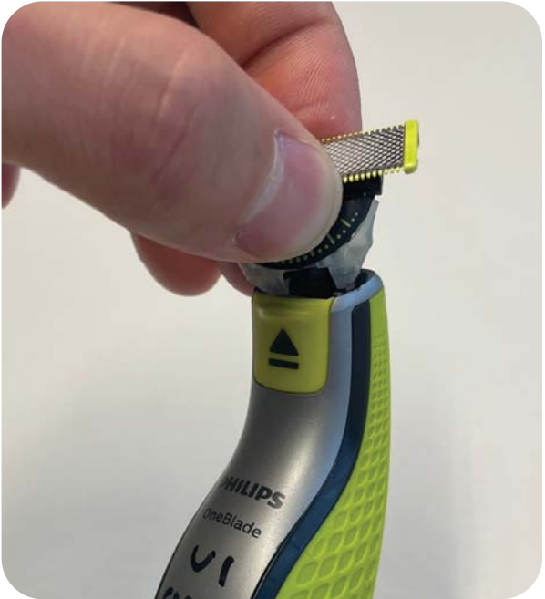
Fig. 95: Detaches with sideways torsion
