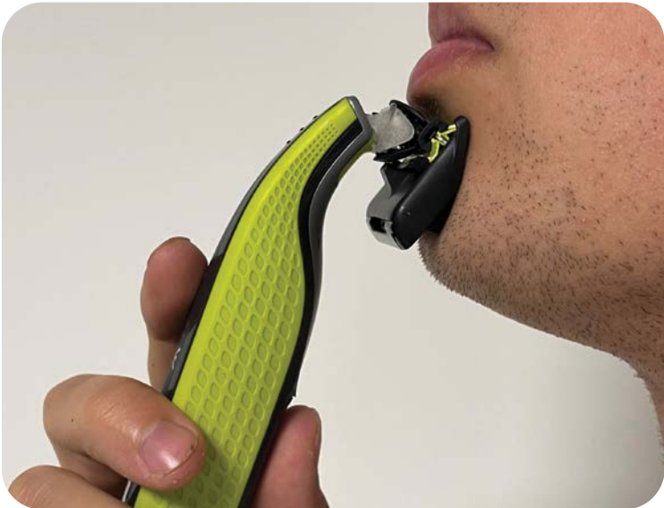
Fig. 115: Just like V2, V3 still detaches with minimal force during shaving.
