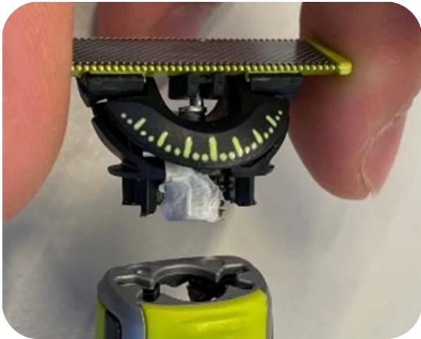
Fig. 80: MVP of the magnetic interface concept: Legs are shortened and the head-power connection is replaced by a magnet, mimicking the concept idea.
