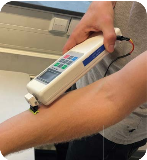
Fig. 52: Measuring the highest F_x on the body
