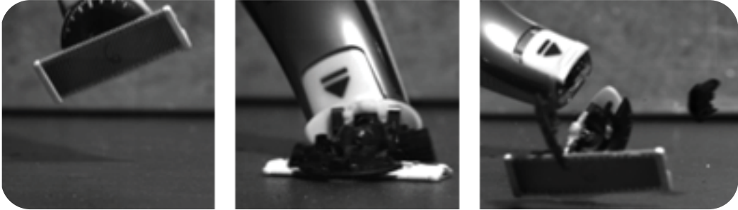
Fig. 102: 70 cm drop on top-side -> Breaks, as after the head detached the handle pushed on the font of the legs, over-rotating the hinge and breaking the front left blade snap-fits.
