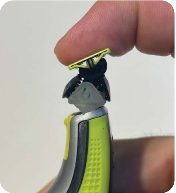
Fig. 94: Detaches with a small frontal moment
