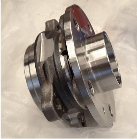
(a) Photo of the modified BAR0282 bearing. Pockets are milled out of the outer ring to create a good surface for the strain gauges to adhere to. There are a total of four of these pockets.
