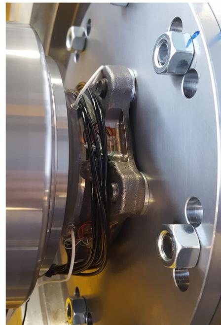
(b) The instrumented bearing installed on BETSY with shims between the outer ring and the plate.
