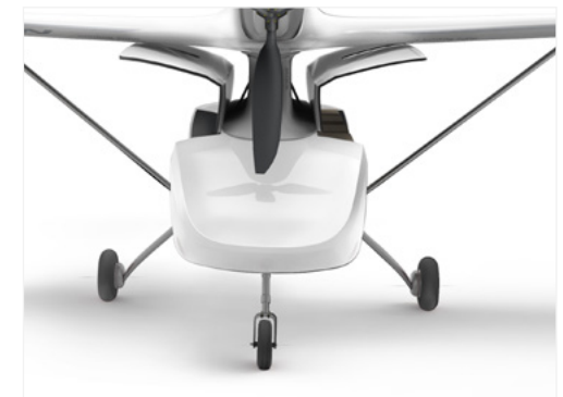
Figure 38 : Protruding wheel and wing strut
