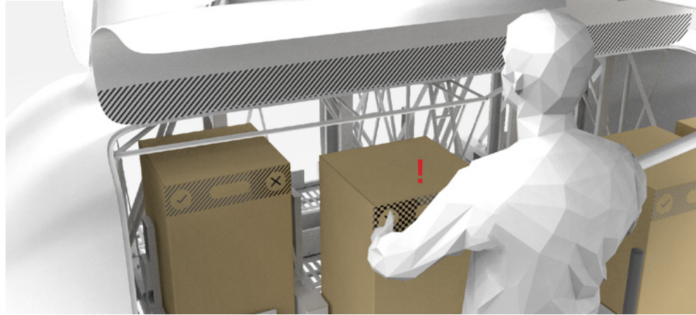
⑦ Boxes are slid into the UAV. Patterns inside the UAV allow verification of correct orientation
