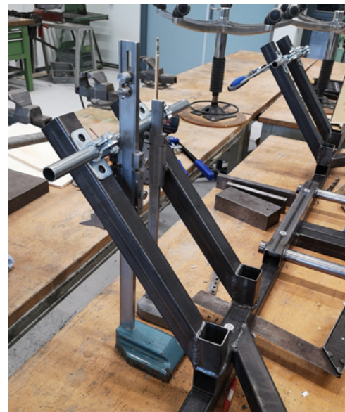
Lining up the wheel axles
