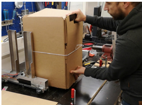
44 Figure 37 : Testing sliding box into cargo bay
