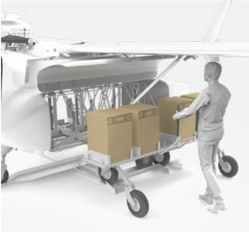
⑥ Loading cart display indicates which side to load. Cart is driven into the alignment rails.
