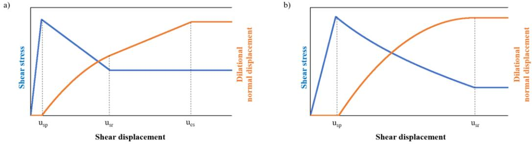
Figure 1. Shear stress-shear displacement and dilational normal displacement caused by shear stress and associated shear displacement for a) Coulomb with softening and b) modified Barton-Bandis models.
