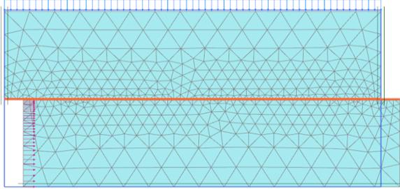
Figure 3. Finite element model for discontinuity shear under CNL conditions.
