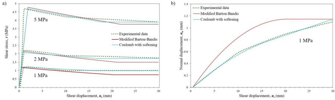
Figure 4. Results of shear CNL tests: (a) shear stress vs. shear displacement, (b) discontinuity dilation.
