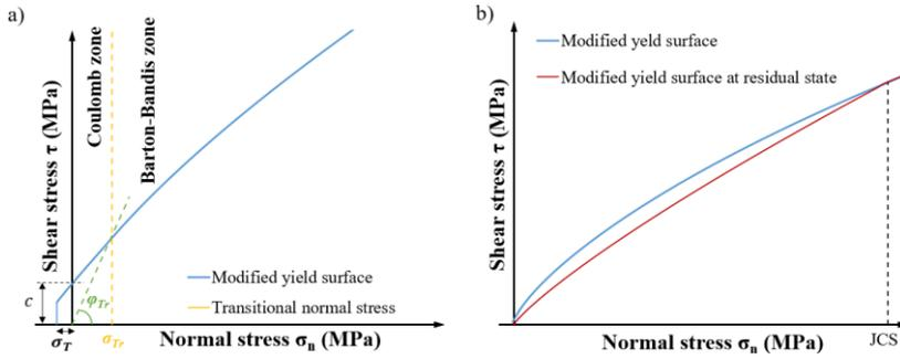
Figure 2. Modified Barton-Bandis model: a) yield surface at low-stress levels; (b) initial/residual envelopes.
