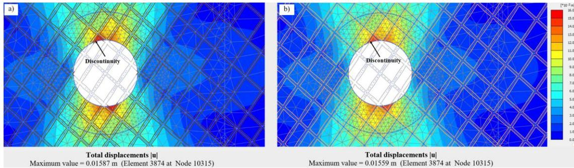
Figure 5. Total displacements: a) modified Barton-Bandis model; b) Coulomb with linear softening.
