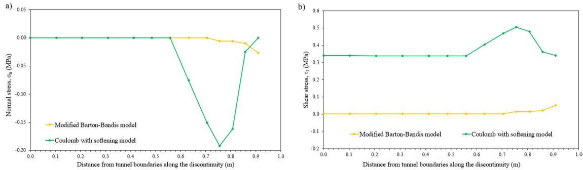
Figure 6. Evolution of a) normal stress and b) shear stress along the discontinuity.
